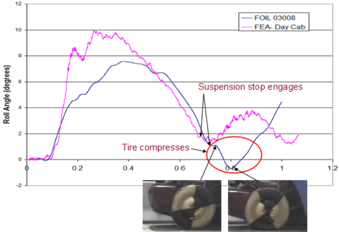
Figure 41. Chart. Roll Angle Measured at the Center of Gravity of the Tractor Showing Annotations from the Tire of the Test Vehicle.
