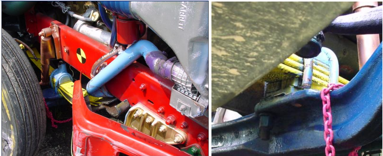
Figure 43. Photograph. Post Test Photos Showing Damage to Suspension Components .
