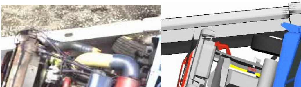
Figure 42. Photograph / Illustration. Snapshot of Test and Simulation Illustrating Primary Load Path between Barrier and Vehicle is through the Bumper and Wheel.
