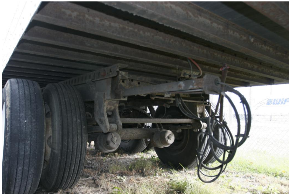
Figure 50. Photograph. Undercarriage of Stoughton Trailer.
