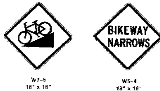
Figure B: Warning signs
