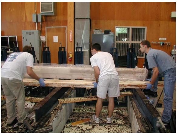
Figure 1: Guardrail Layup in Progress
