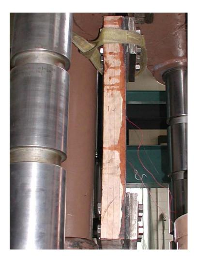
Figure 2: Rail Tension Splice Test
