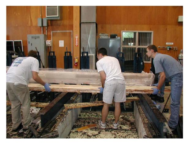
Figure 1: Guardrail Layup in Progress
