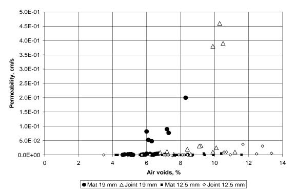
Figure 4. Plot of air voids versus permeability
