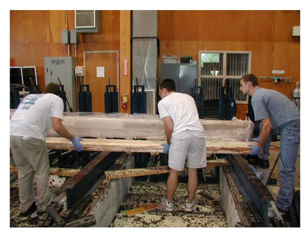
Figure 1: Guardrail Layup in Progress
