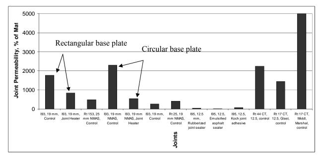
Figure 2. Permeability of different joints, as percentage of permeability of mats
