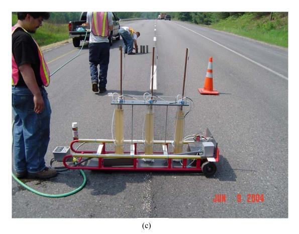
Figure 1. (a) Permeameter taken down from truck; (b) Filling with water; (c) close-up of permeameter on joint
