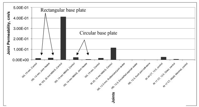
Figure 3. Permeability of different joints
