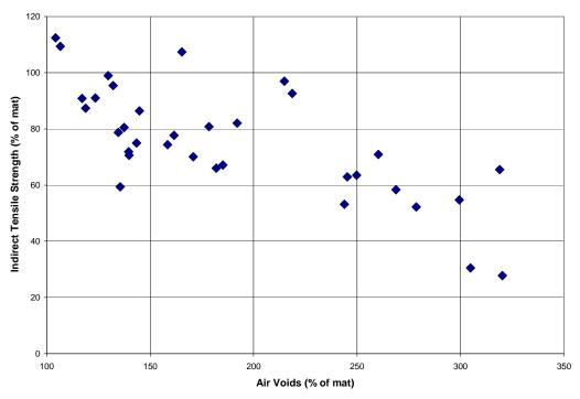
Figure 5. Plot of air voids versus indirect tensile strength of joints
