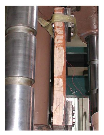
Figure 2: Rail Tension Splice Test
