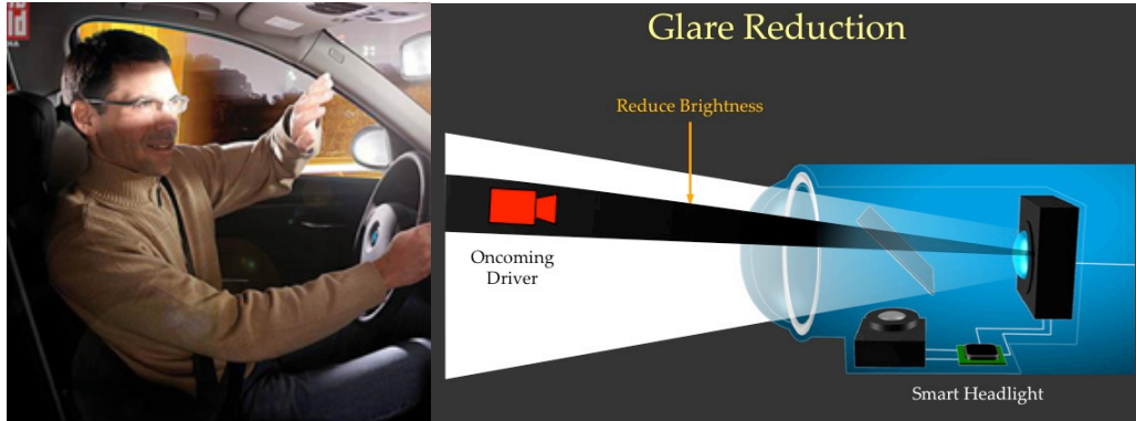
Figure 5: Illustrating the problem and solution for glare from headlights. Glare can cause temporary blindness when driving that can lead to catastrophic accidents. The smart headlight system identifies the oncoming drivers and reduces the intensity to a small region covering each driver on the road. The driver of the smart headlight enabled vehicle is then free to use high beams potentially all the time without worrying about switching them.
