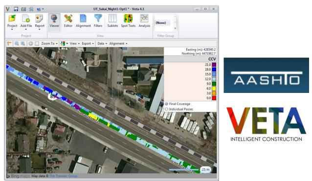
Figure 7. AASHTO Standard Software Veta for Intelligent Construction Data Management.
