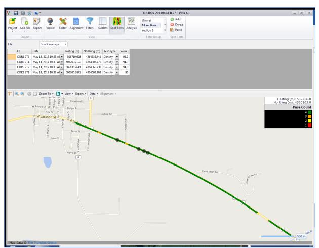
Figure 42: An Example Veta Analysis Screen showing spot tests (J1P3005 RT 24).
