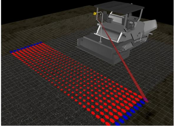
Figure 5. An Illustration of an IR System.
