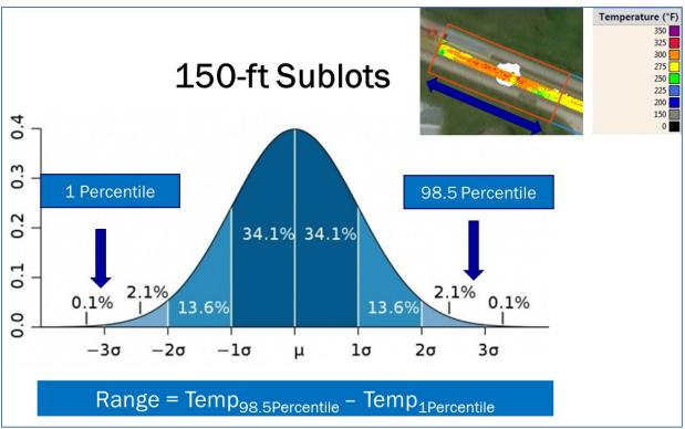
Figure 22: AASHTO PP80 IR Analysis Method: Computation of "Range" value
