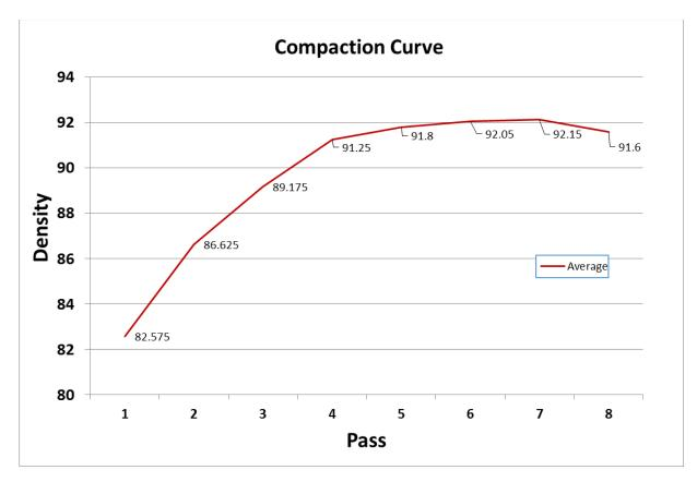
Figure 54 Compaction Curve SP095B from the Trial Section on8/26/2017 (Project No. 2 - J4I3111, RT 29).
