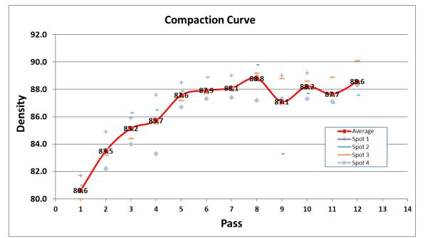
Figure 49 Compaction Curve from the Trial Section on 5/12/2017 (Project No. 1 - J5P3117, RT 52).
