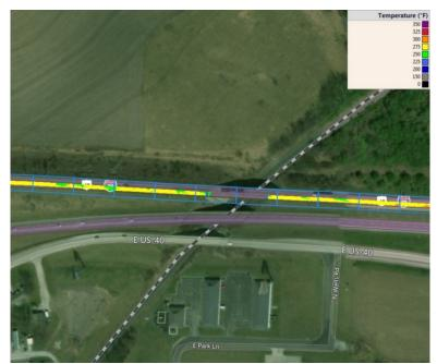
Figure 28: Example of a Veta Sublot screen for IR data analysis (J3I3042, RT70).
