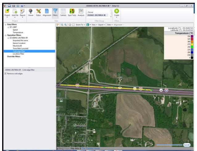
Figure 26: Example of Veta Filter screen (J3I3042, RT70).
