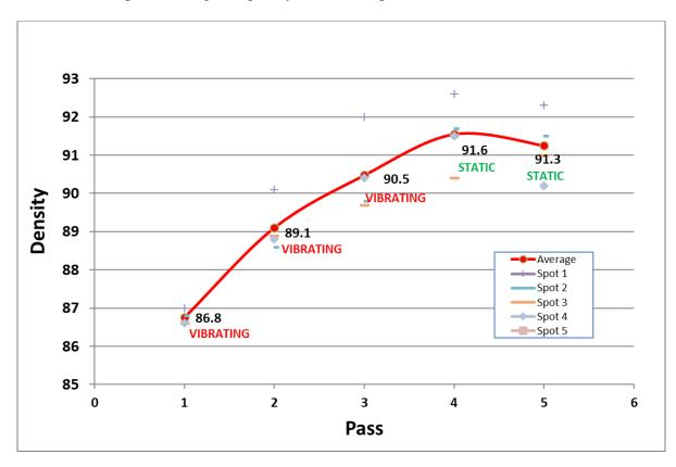
Figure 77: Compaction Curve– Trial Section (4/24/2017) (Project No. 7 - J1P3005, RT 24)
