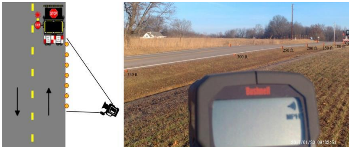
Figure 2.1.1 Field Study Plan of Cameras, Radar Speed Gun, and Delineators
