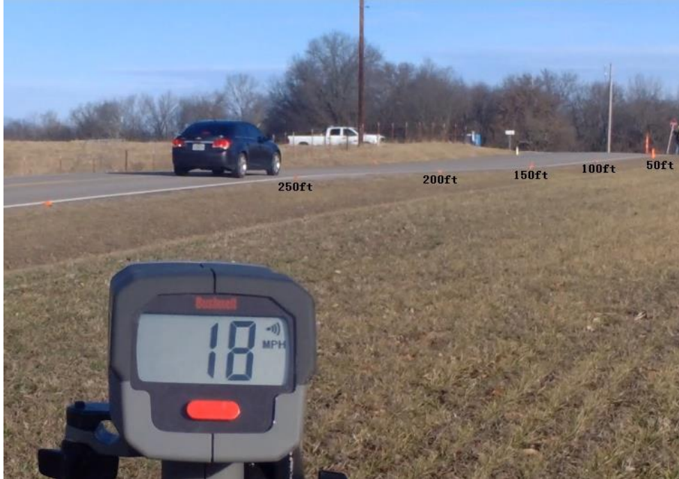
Figure 2.3.4 MOE 1 Example: Speed of the Leading Vehicle at 250 ft. from AFAD/Flagger
