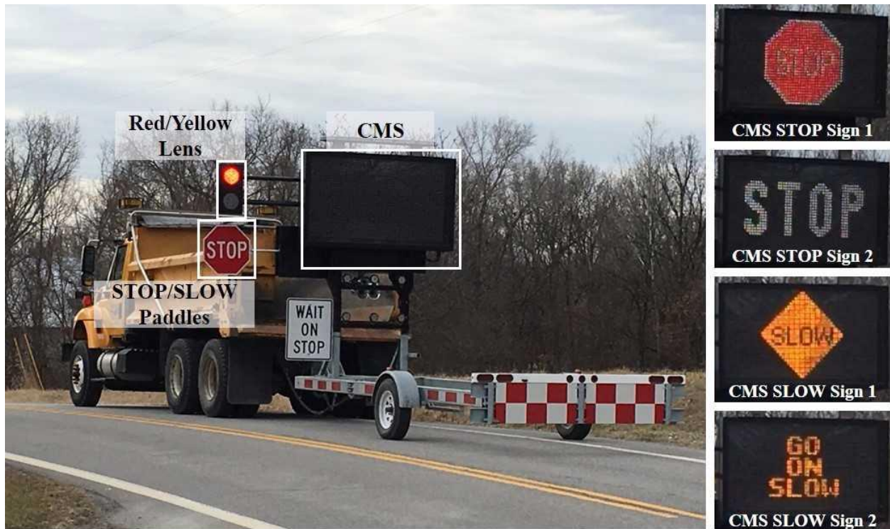
Figure 1.1.1 AFAD Mounted on TMA
