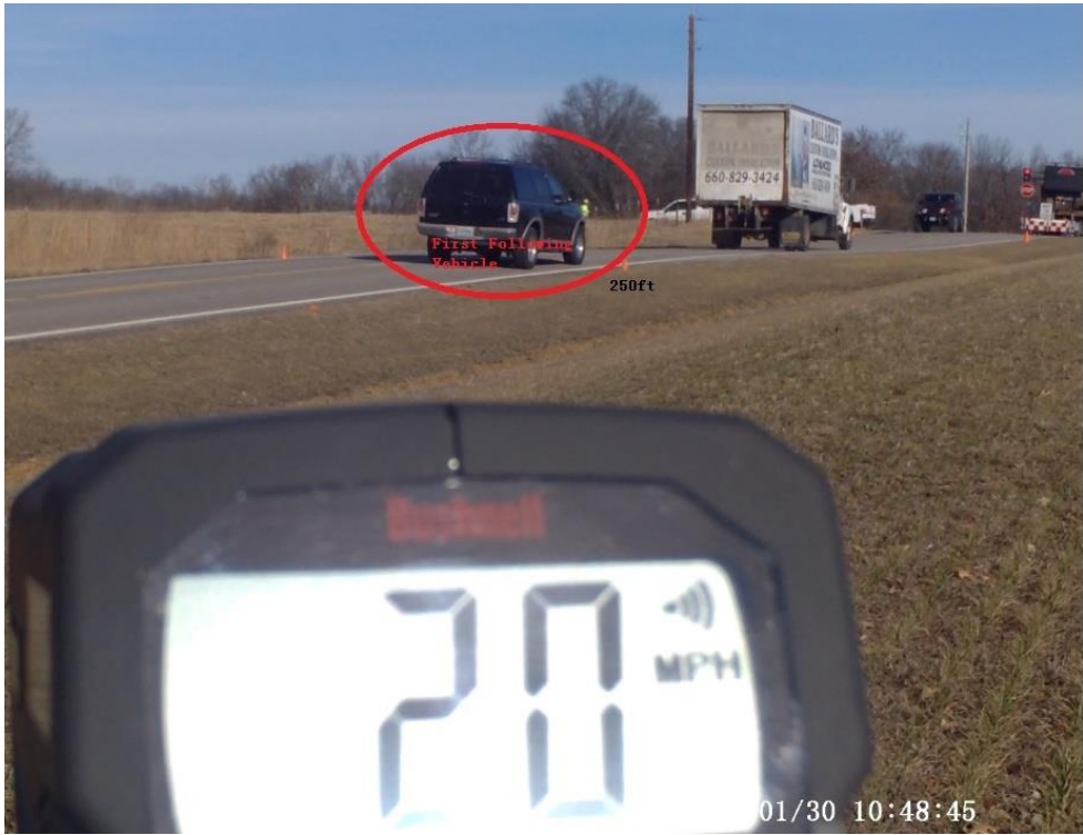
Figure 2.3.9 MOE 6: Speed of the 1st Following Vehicle at 250 ft. from AFAD/Flagger
