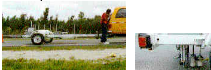
Figure 2-3: Seismic Pavement Analyzer (SPA)
