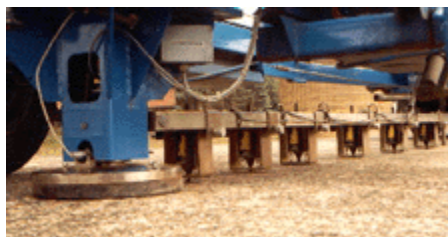
Figure 2-2: FWD Load Plate and Sensors
