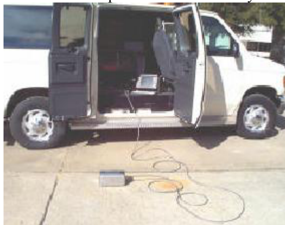
Figure 2-4: Portable Seismic Pavement Analyzer (PSPA)
