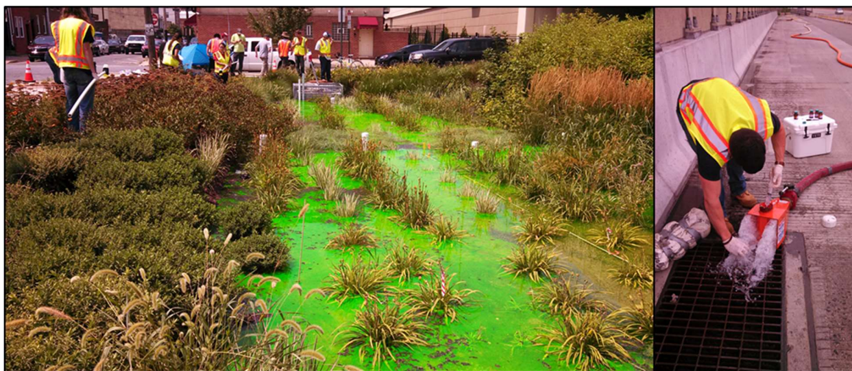
Figure 4-2. Left panel: fluorescein in SMP C. Right panel: near-continuous addition of LiBr.
