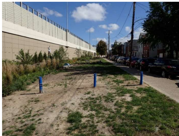
Figure 3-19: Wells with Decagon CTD-10 Pressure Transducers
