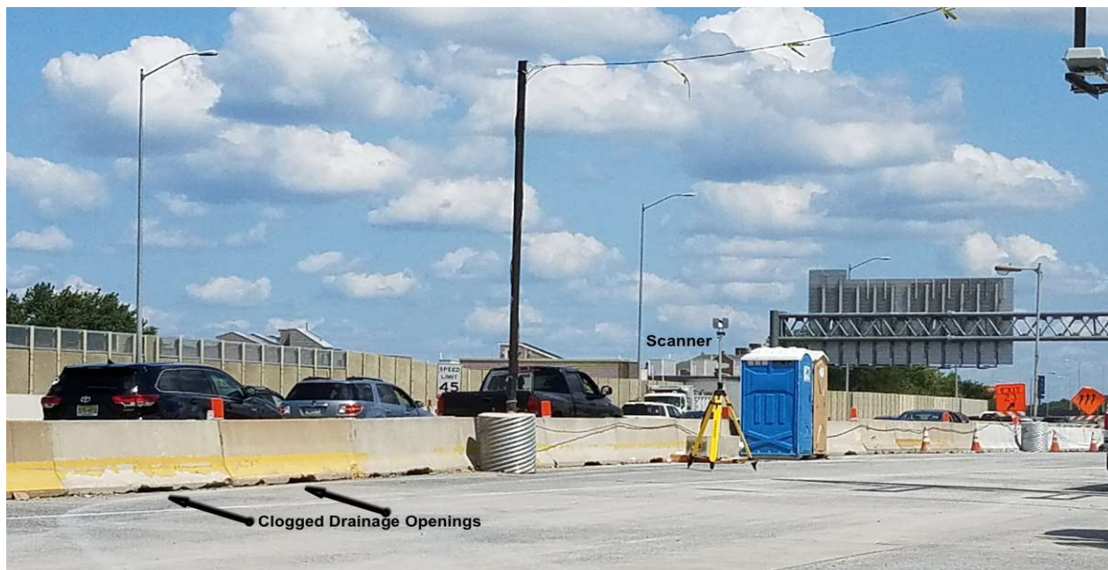
Fig. 5.10 Photograph showing the LiDAR scanner, concrete barriers, and their drainage openings.
