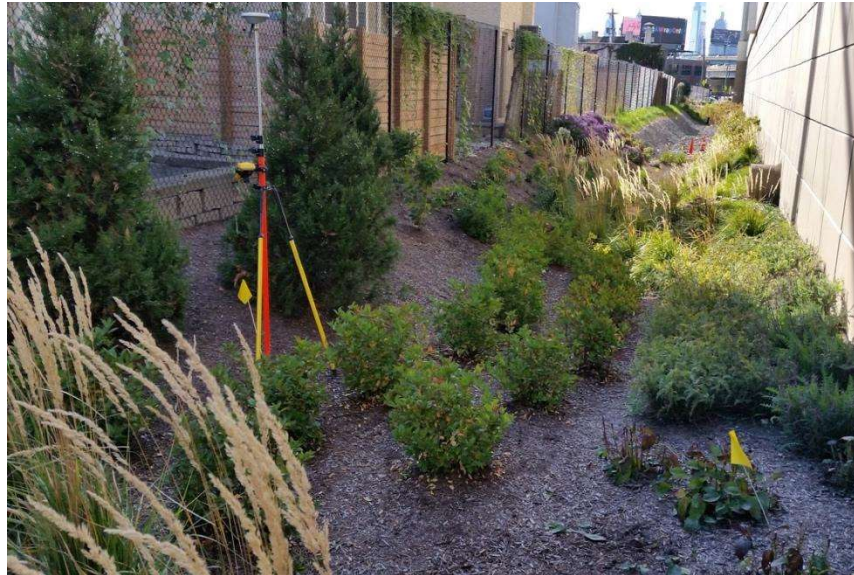
Fig. 5.2. The Trimble Geo XH GPS used to georeference the LiDAR-derived point cloud data.
