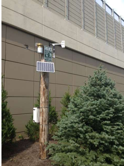
Figure 3-8. Weather station installed between SMPs C and D.
