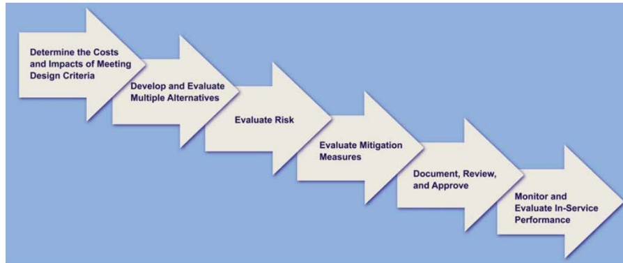
Figure 2: Illustration of the Federal Highway Administration Design Exception Process; Adopted from Mitigation Strategies for Design Exceptions (Stein & Neuman, 2007)
