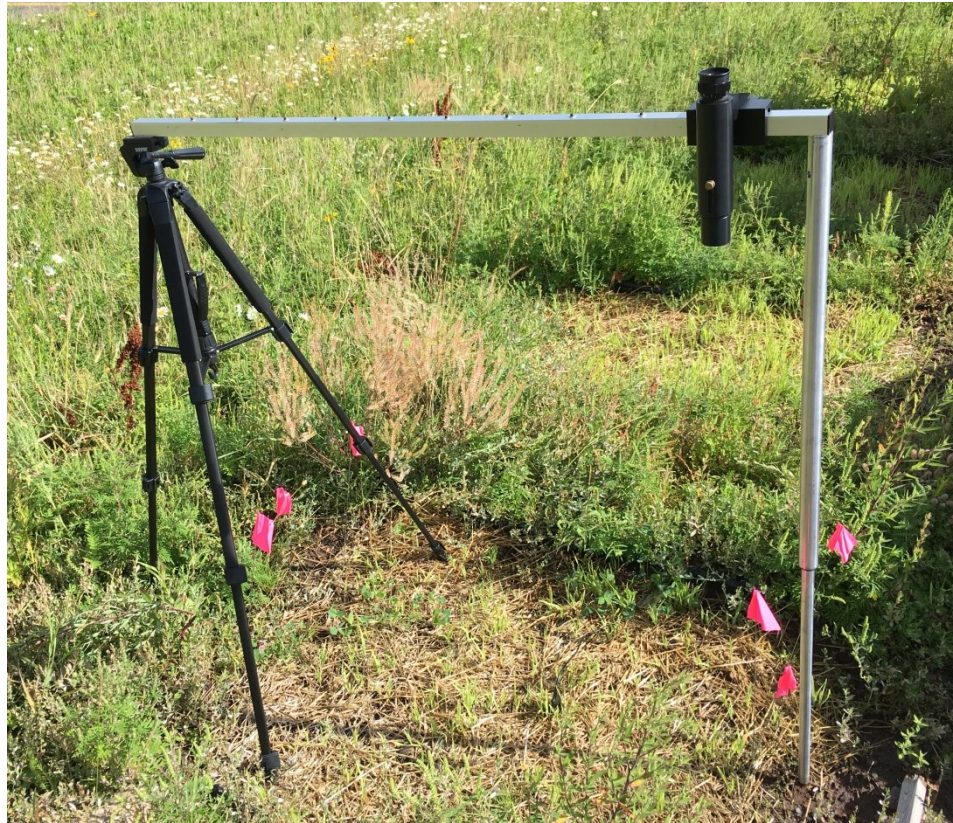
Figure 6.17 Cover-Point Optical Device used to determine percent plant cover.
