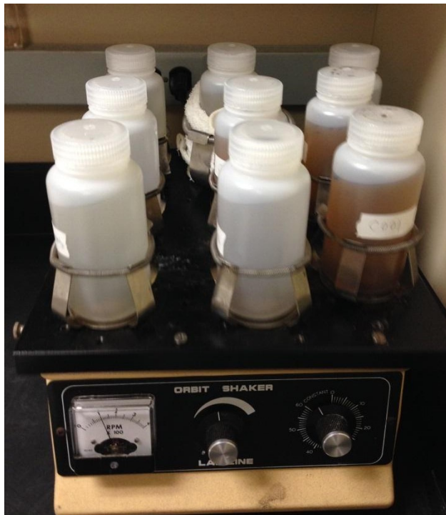
Figure 4.2. Mixture of synthesized stormwater and filtration materials was being shaken at 100 rpm.
