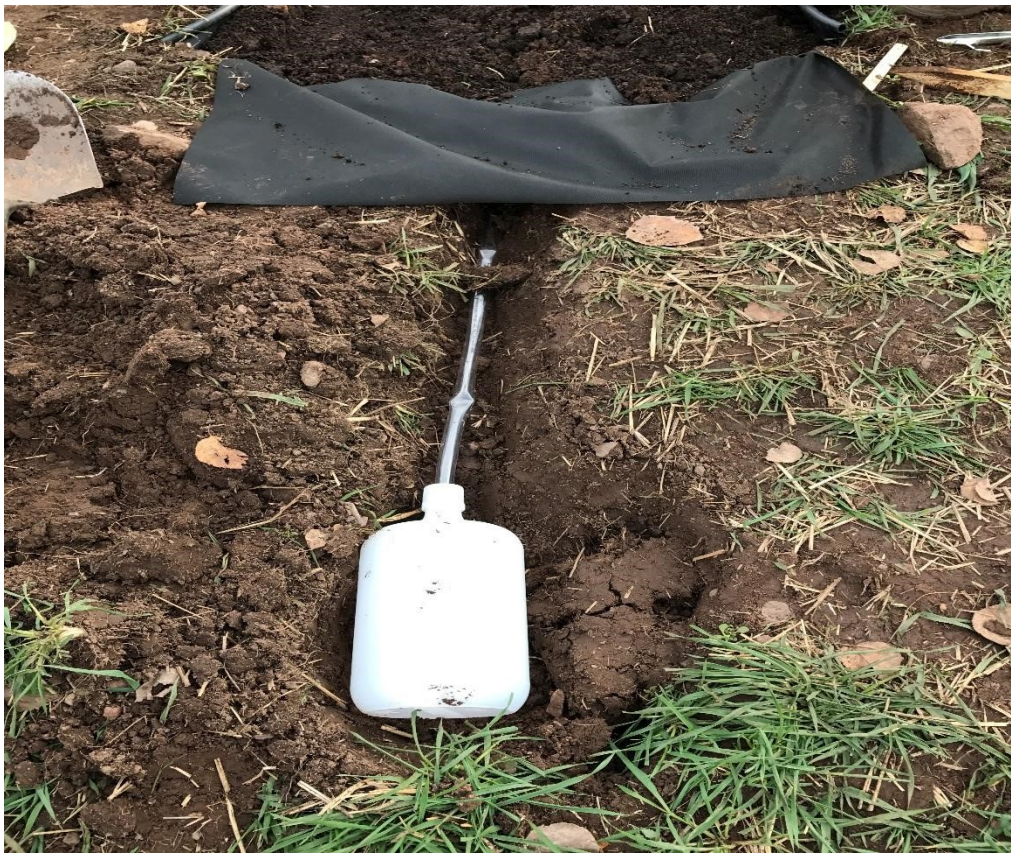
Figure 6.4 Effluent water collection vessel for water quality analysis.
