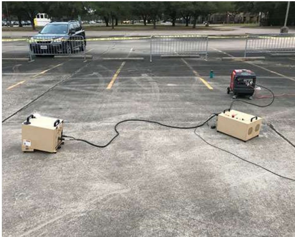
Figure 5. Tethered UAS Setup with Generator, Power Regulator, and Spooler
