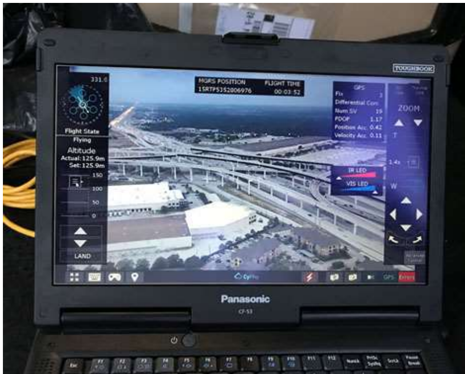
Figure 7. Tethered Flight Control Software with Incorporated Video
