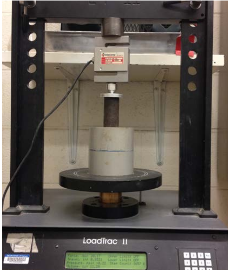
Figure 3.8: Standard Setup for Unconfined Compression Strength Test
