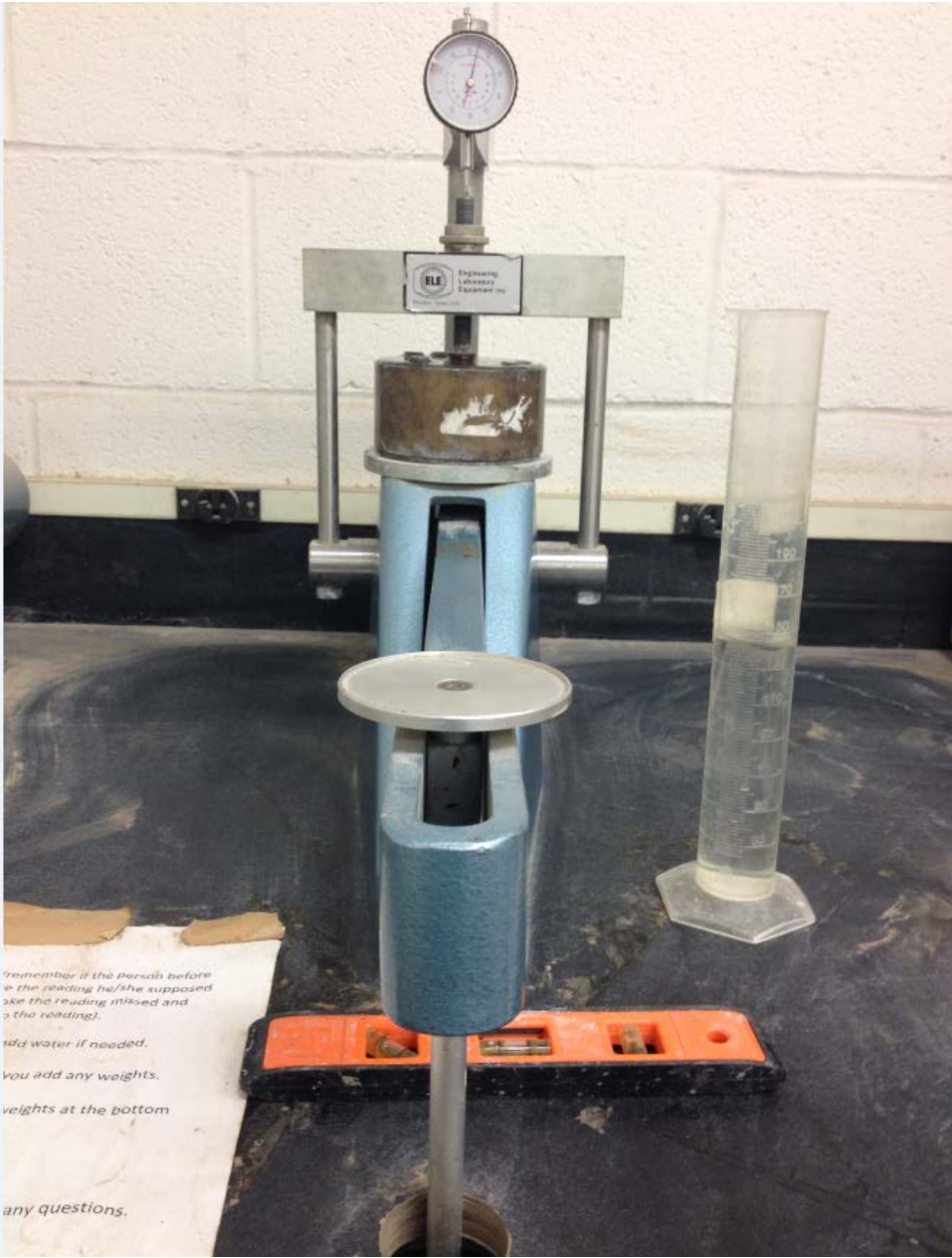
Figure 3.6: Swell Test Setup
