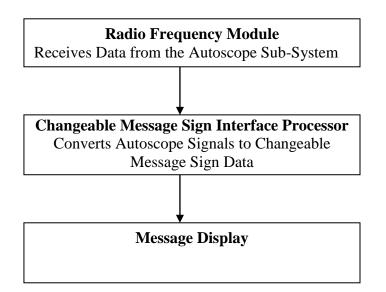
Figure B10 Changeable Message Sign Sub-System Operation Flow
