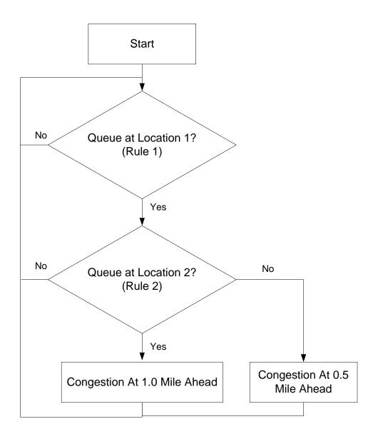
Figure B12 Control Logic for Displaying Messages on a Changeable Message Sign
