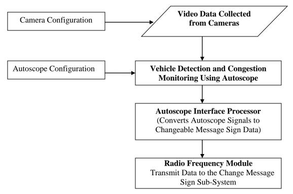
Figure B8 Autoscope Sub-System Operation Flow
