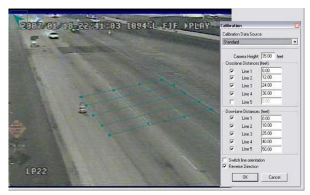
**Figure 4.3 Calibration of Autoscope**
