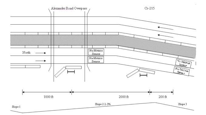
Figure 3.6 Layout of Speed Trailer and Detectors on the Test Site on Cr-215
