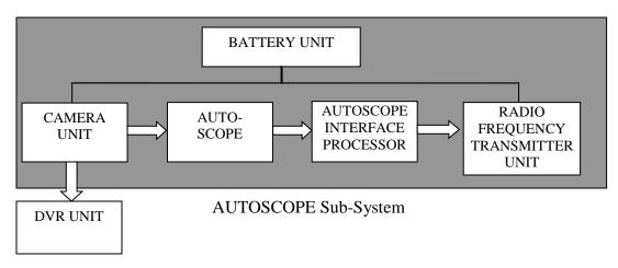
Figure B7 Autoscope Sub-System Block Diagram
