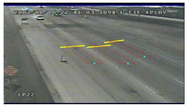
**Figure 4.5 Speed Detector**
