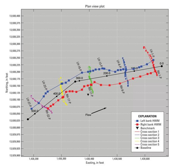
**Figure 3.** Plan view of the site showing the left and right bank high-water marks (HWMs) and cross sections for Big Cottonwood Creek at U.S. Highway 50 near Coaldale, Colorado; generated using the Slope-Area Computation Graphical User Interface. For readability, not all data points are labeled.
