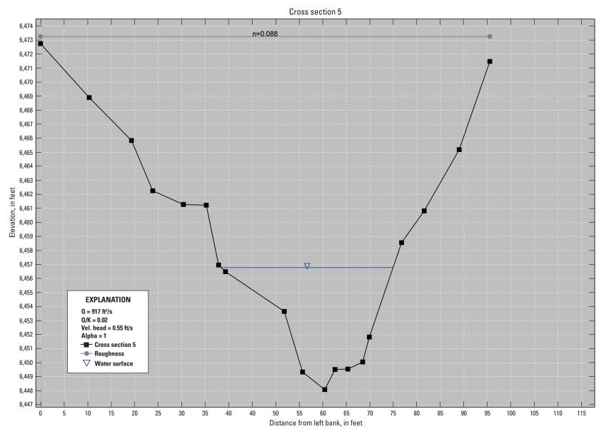
**Figure 5-5.** Cross section 5 with the Manning roughness coefficient (n) assignment for Big Cottonwood Creek at U.S. Highway 50 near Coaldale, Colorado; generated from the Slope-Area Computation Graphical User Interface. [X5, cross section 5; Q, discharge; ft<sup>3</sup>/s, cubic foot per second; K, conveyance; Vel., velocity; ft/s, foot per second]
