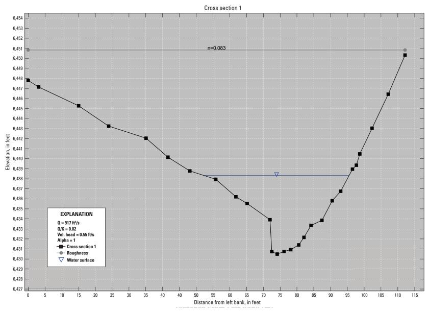
**Figure 5-1.** Cross section 1 with the Manning roughness coefficient (n) assignment for Big Cottonwood Creek at U.S. Highway 50 near Coaldale, Colorado; generated from the Slope-Area Computation Graphical User Interface. [X1, cross section 1; Q, discharge; ft<sup>3</sup>/s, cubic foot per second; K, conveyance; Vel., velocity; ft/s, foot per second]
