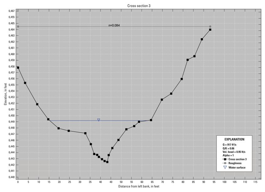
**Figure 5-3.** Cross section 3 with the Manning roughness coefficient (n) assignment for Big Cottonwood Creek at U.S. Highway 50 near Coaldale, Colorado; generated from the Slope-Area Computation Graphical User Interface. [X3, cross section 3; Q, discharge; ft<sup>3</sup>/s, cubic foot per second; K, conveyance; Vel., velocity; ft/s, foot per second]
