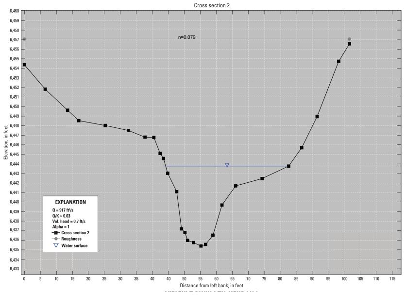
**Figure 5-2.** Cross section 2 with the Manning roughness coefficient (n) assignment for Big Cottonwood Creek at U.S. Highway 50 near Coaldale, Colorado; generated from the Slope-Area Computation Graphical User Interface. [X2, cross section 2; Q, discharge; ft<sup>3</sup>/s, cubic foot per second; K, conveyance; Vel., velocity; ft/s, foot per second]
