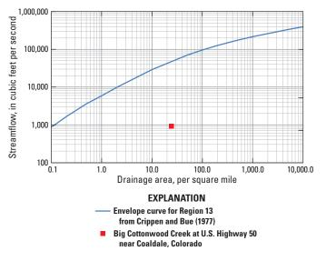
**Figure 7.** The envelope curve for Region 13 from Crippen and Bue (1977) with the flood of August 23, 2016, on Big Cottonwood Creek at U.S. Highway 50 near Coaldale, Colorado.
