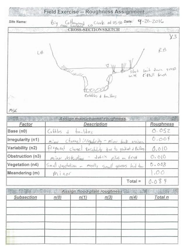
**Figure 4-3.** The Manning roughness coefficient (n) assignment for cross section 3 on Big Cottonwood Creek at U.S. Highway 50 near Coaldale, Colorado.
