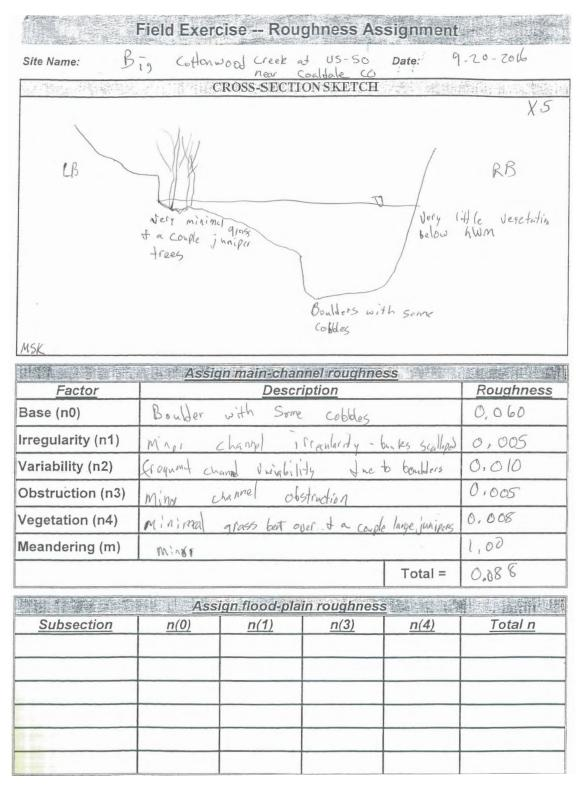
**Figure 4-5.** The Manning roughness coefficient (n) assignment for cross section 5 on Big Cottonwood Creek at U.S. Highway 50 near Coaldale, Colorado.
