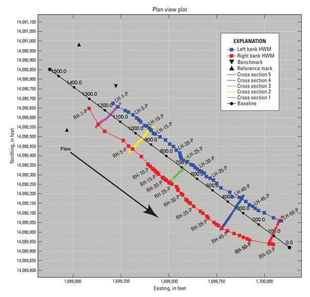
**Figure 10.** Plan view of the site showing the left and right bank high-water marks (HWMs) and cross sections for Fountain Creek below U.S. Highway 24 in Colorado Springs, Colorado; generated from the Slope-Area Computation Graphical User Interface. For readability, not all data points are labeled.
