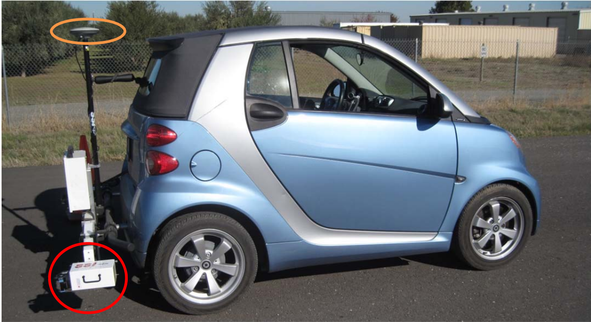
Figure 3.13: SSI lightweight inertial profiler with rear-mounted high-speed lasers, one in each wheelpath (red circle, shows laser in right wheelpath) and GPS unit (orange oval).
