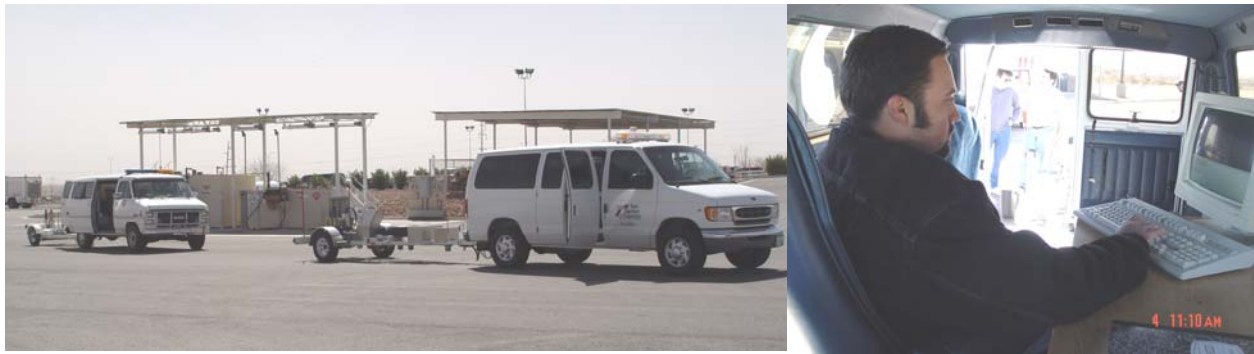
Figure 4.2 - FWD and SPA Devices in Operation at TxDOT Parking Lot (El Paso)
