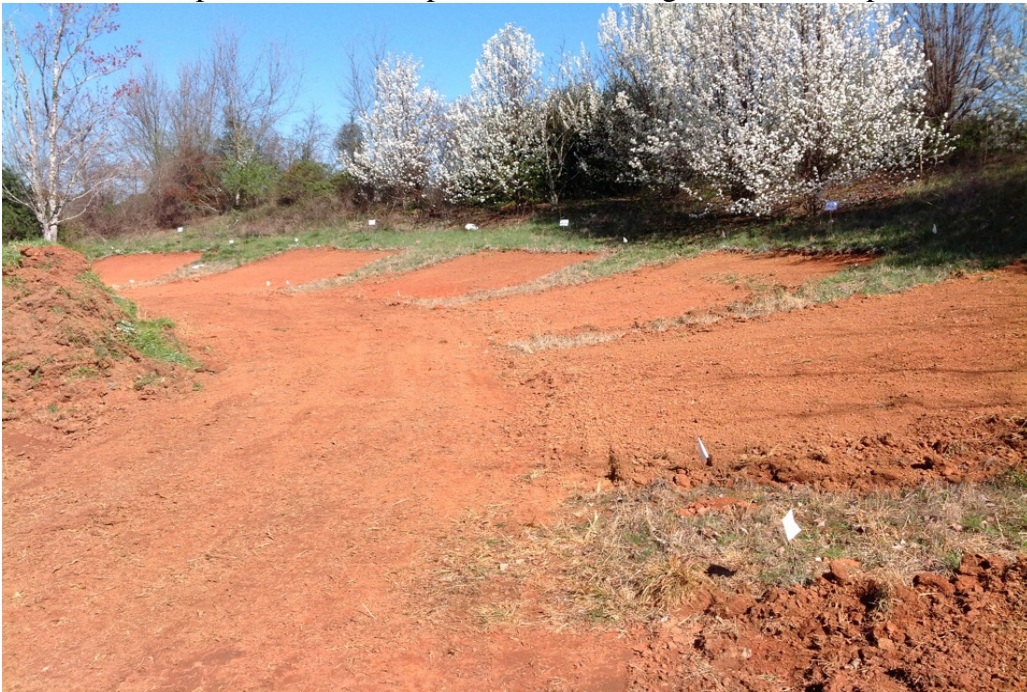
Picture 2. A replication in the experiment consisting of the four slope ratios evaluated.
