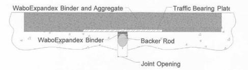
Physical Properties: Elastomeric Binder Modified elastomeric binder shall meet or exceed the requirements of ASTM-3405 and ASTM-1190.
