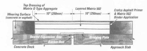
Figure 1. Typical Matrix 502 Asphaltic Plug Bridge Joint System
