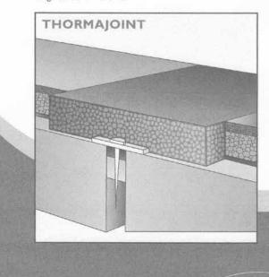
All joints extend the full depth of the asphalt road surfacing and waterproof membrane down to the deck concrete. In certain instances the engineer may decide that a rebate may be created in the concrete, to increase the depth of the joint to the required dimension (table 1).
