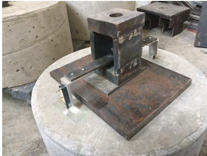
Figure 4.19: Linear potentiometers attached to steel bar
