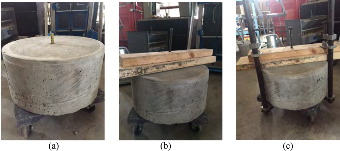
Figure 4.9: Installation setup for adhesive in glass capsule format
