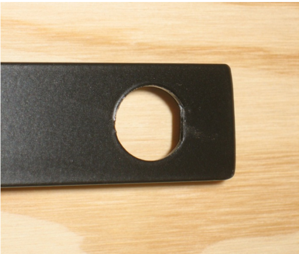
Figure 27. Photo. 5/8" "D" antenna mounting hole.
