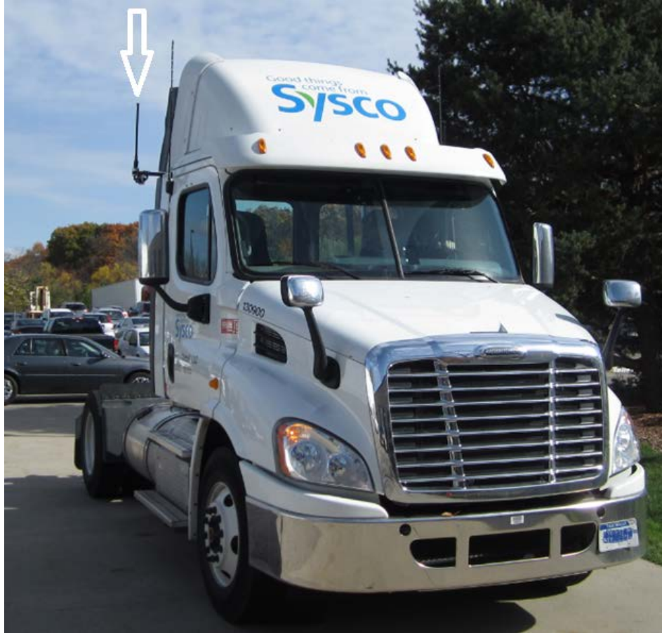
Figure 6. Photo. Front view of a tractor with the RSD kit installed. The arrow points to the right-side DSRC antenna. This tractor was outfitted for the Model Deployment.
