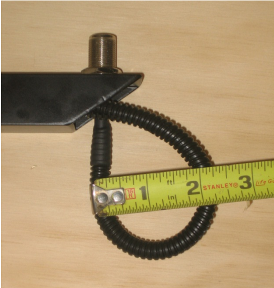
Figure 29. Photo. RF cable loop.
