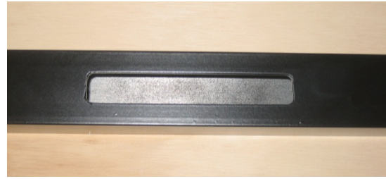
Figure 30. Photo. 4" slot cutout.
