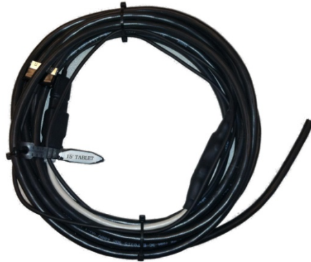
Figure 44. Photo. Tablet power cable.
