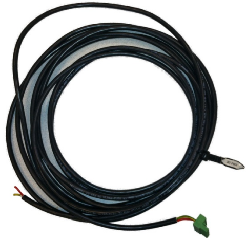
Figure 39. Photo. Access point power cable.
