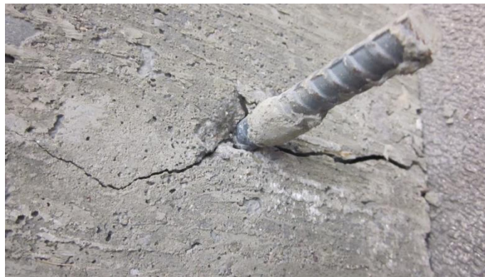
Figure 28: Failure Mode of a Push Through Bond Strength Control Specimen
