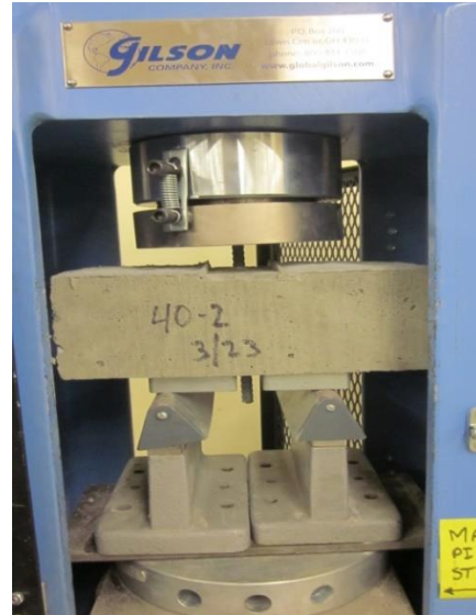
Figure 10: Testing Set-up for Bond Strength Push Through Test
