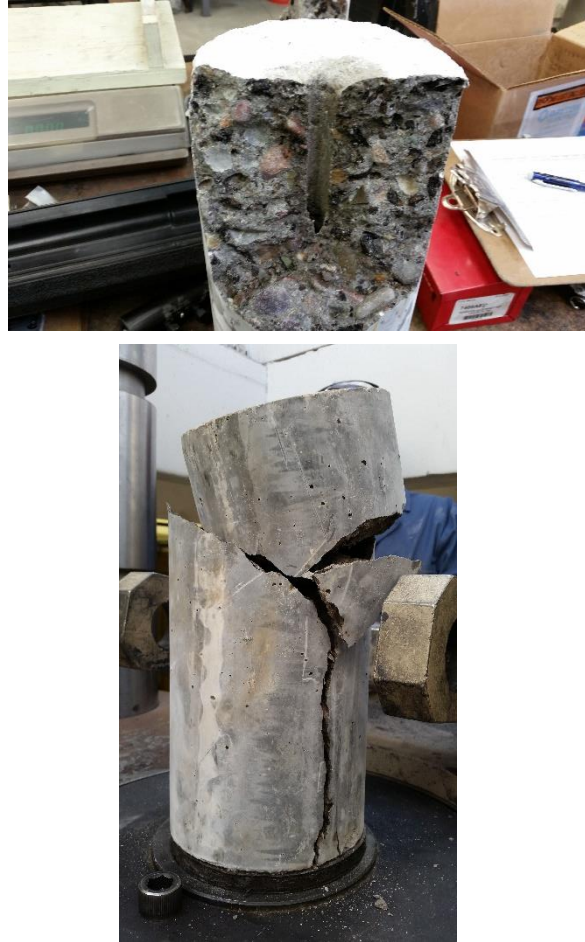
Figure 29: Pull Out Bond Strength Testing Failure Modes (Mode 1 Top, and Mode 2 Bottom)
