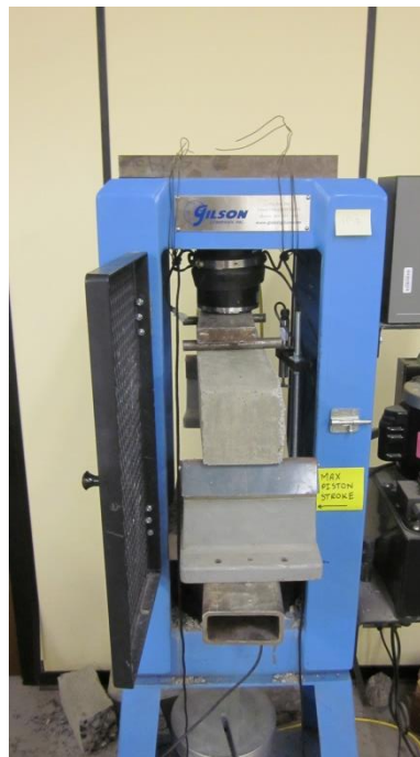
Figure 13: Test Set-up for Ductility Test
