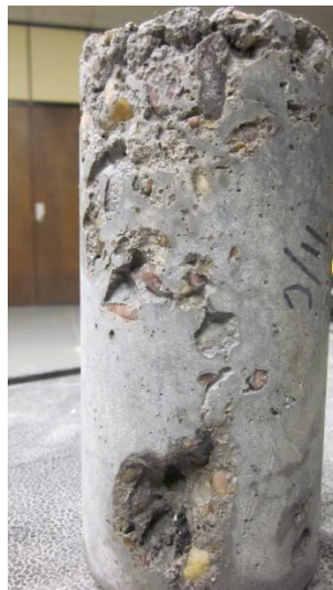
Figure 24: 25 Percent RAP After 108 Freeze-Thaw Cycles
