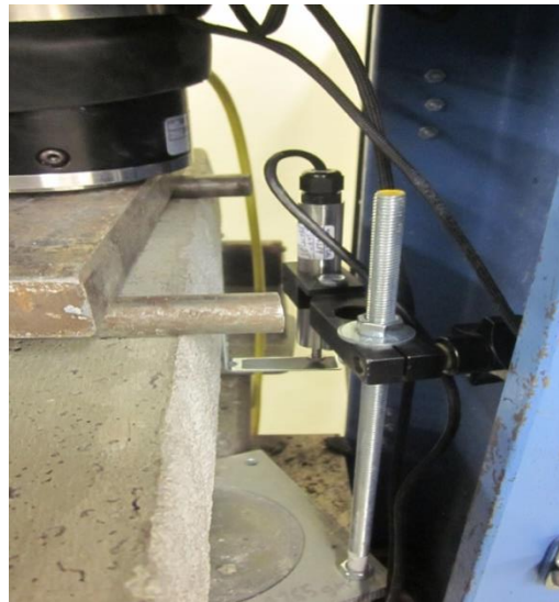
Figure 14: LSCT Set-up for Ductility Testing
