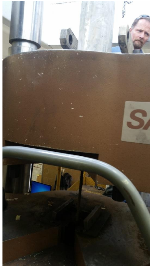
Figure 11: Testing Set-up for Bond Strength Pull Out Test
