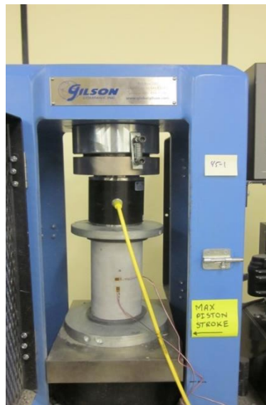
Figure 16: Test Set-up for Strain Rate Test
