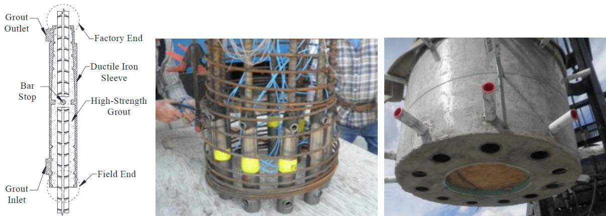
Figure 3. Grout-filled Sleeve Coupler and Placement in the GCNP Column (1)
