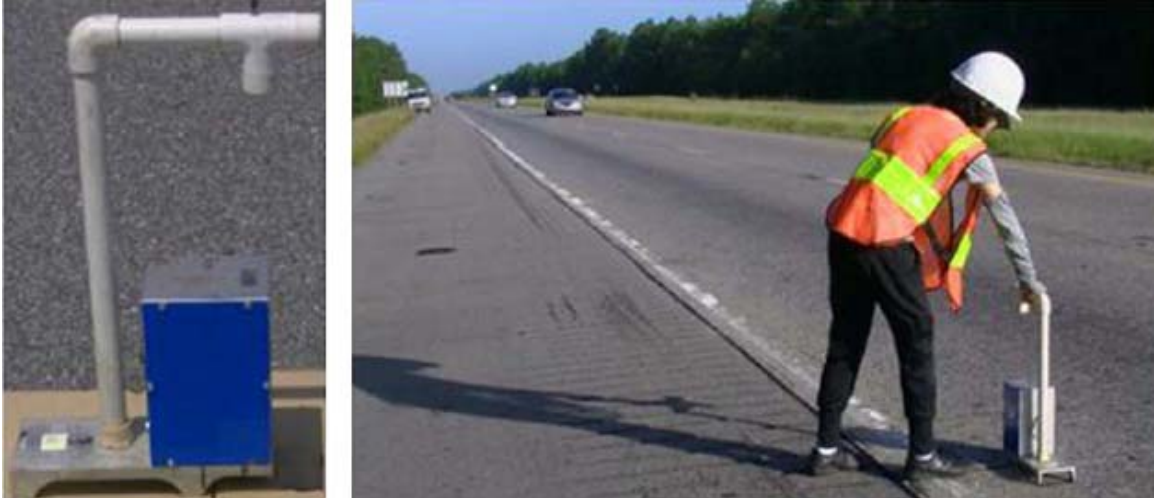
FIGURE 3.27: Left: Georgia Faultmeter; Right: Manual measurement on the roadway
