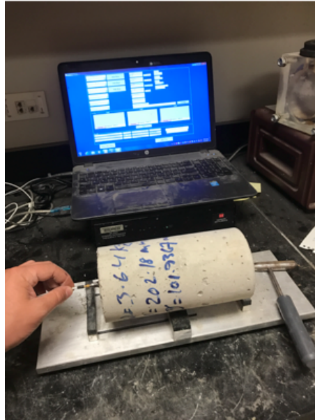
Figure 6-27. Dynamic Modulus of Elasticity Test Configuration
