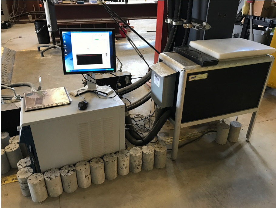
Figure 6-31. Coefficient of Thermal Expansion Test Equipment.
