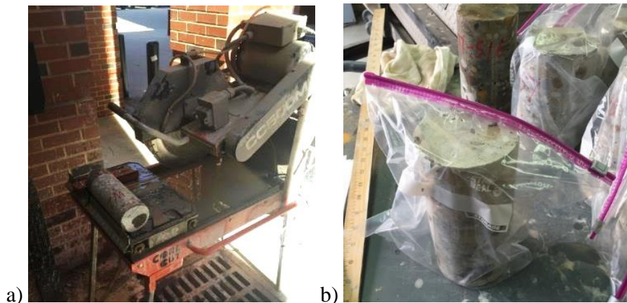
Figure 11 a) Saw used in core preparation; b) Core specimen in a sealed bag for moisture conditioning.
