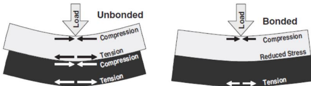
Figure 4 Comparison of overlay strain profiles: a) unbonded; b) bonded [Kivi et al., 2013].
