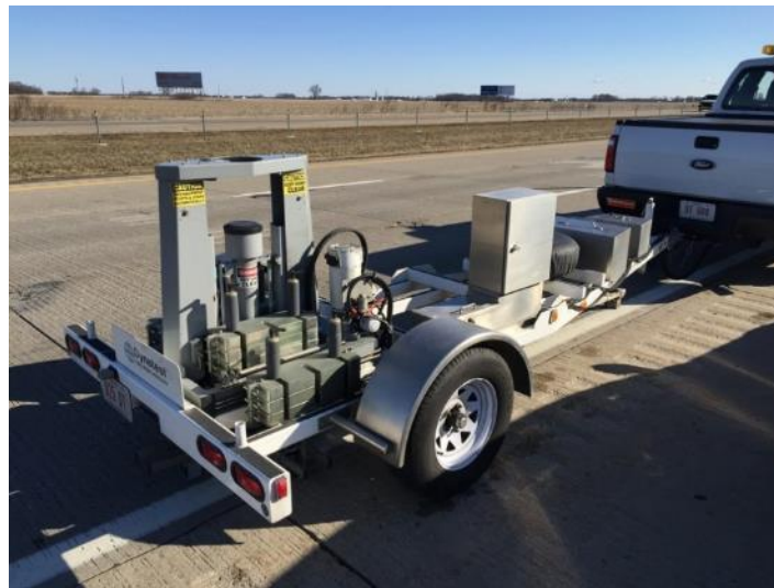
Figure 6 FWD used by ODOT
