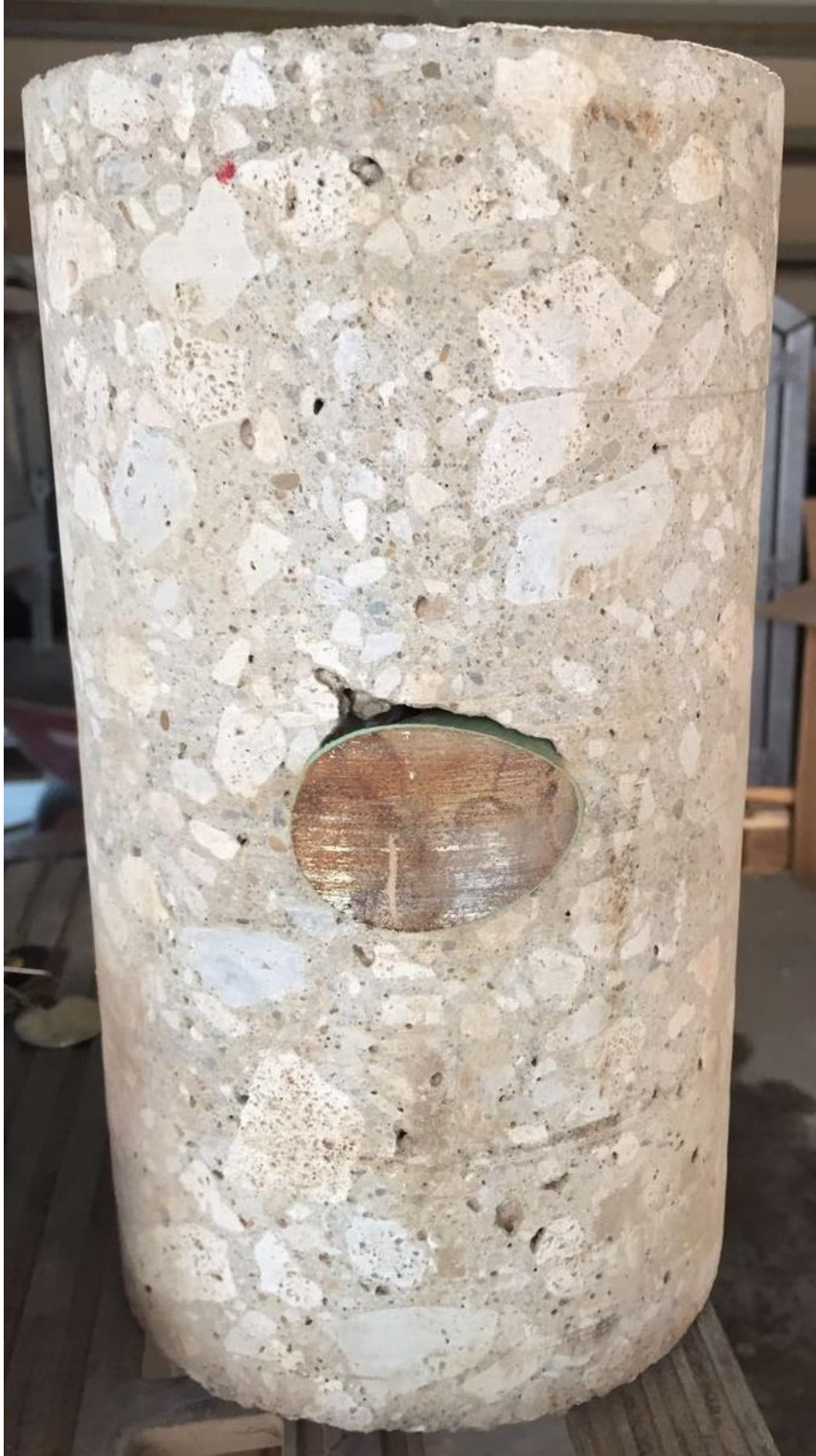
Figure 66 Uncut tangential core form WAY-30 showing gap above dowel bar.
