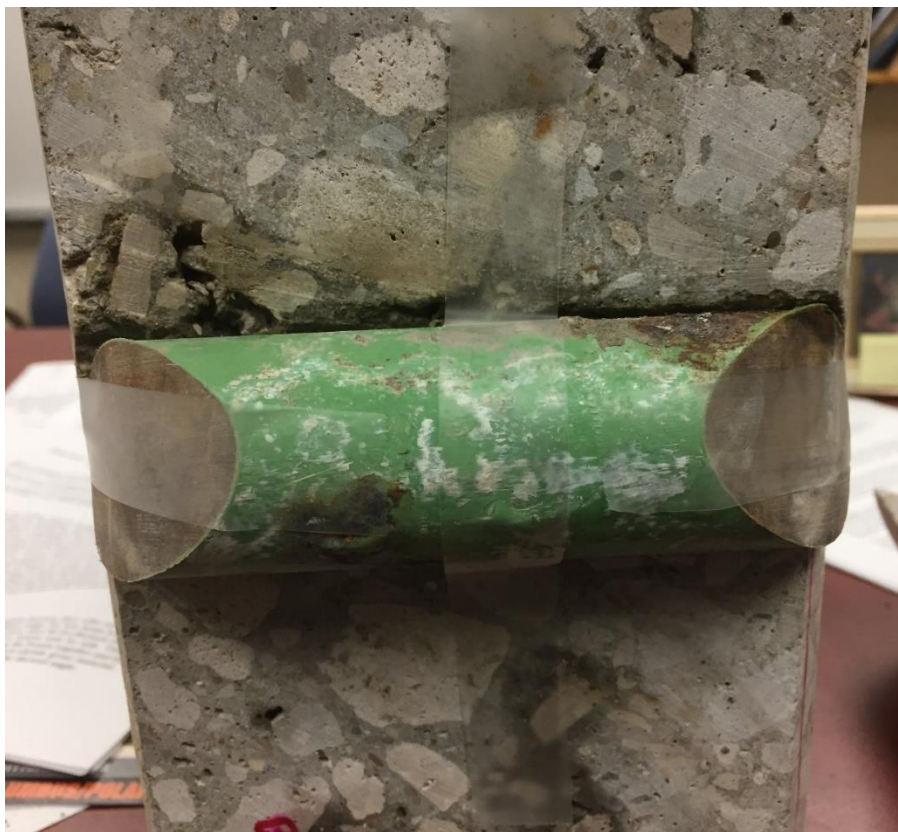
Figure 68 Close-up of tangential core from WAY-30 showing space above dowel bar and some entrapped air voids. Note that the dowel bar is held in place with clear adhesive tape.
