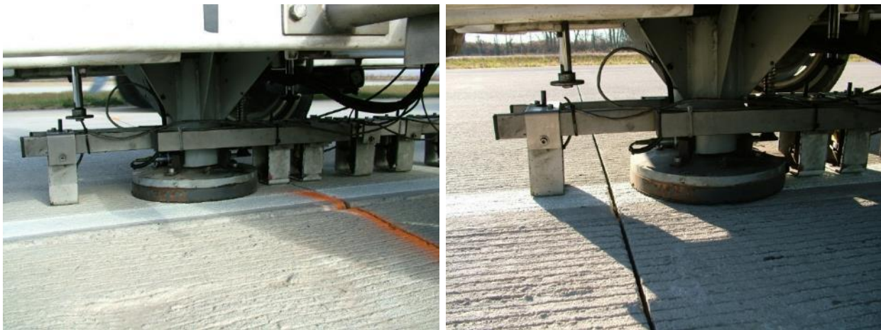
Figure 8 a) Joint approach position; b) Joint leave position. Note that sensor cradle immediately to right of the load plate is empty.
