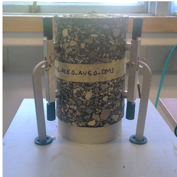
Figure 3.19: Gauge point gluing setup
