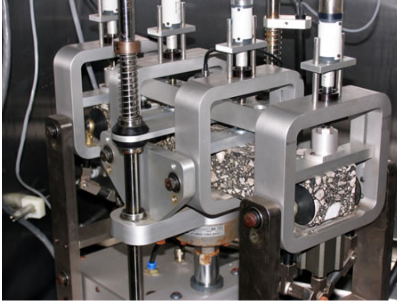
Figure 2.7: Four-point bend testing system (Source: www.pavementinteractive.org ).
