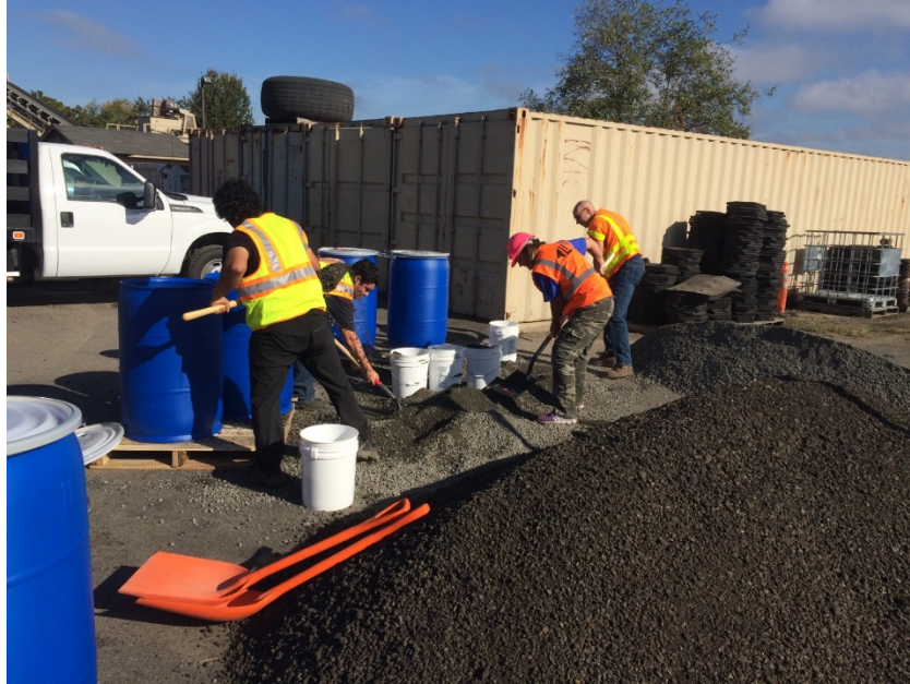
Figure 3.1: Asphalt mix sampling at the production plant.
