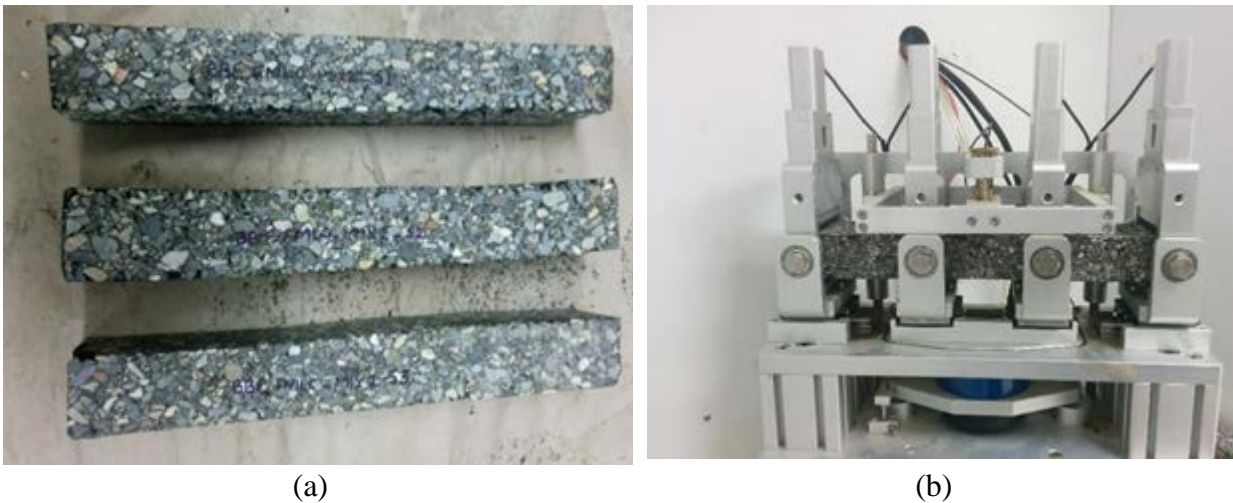
Figure 3.14: Bending beam fatigue test; (a) Beam specimens prepared with roller compactor; (b) four-point bending test apparatus
