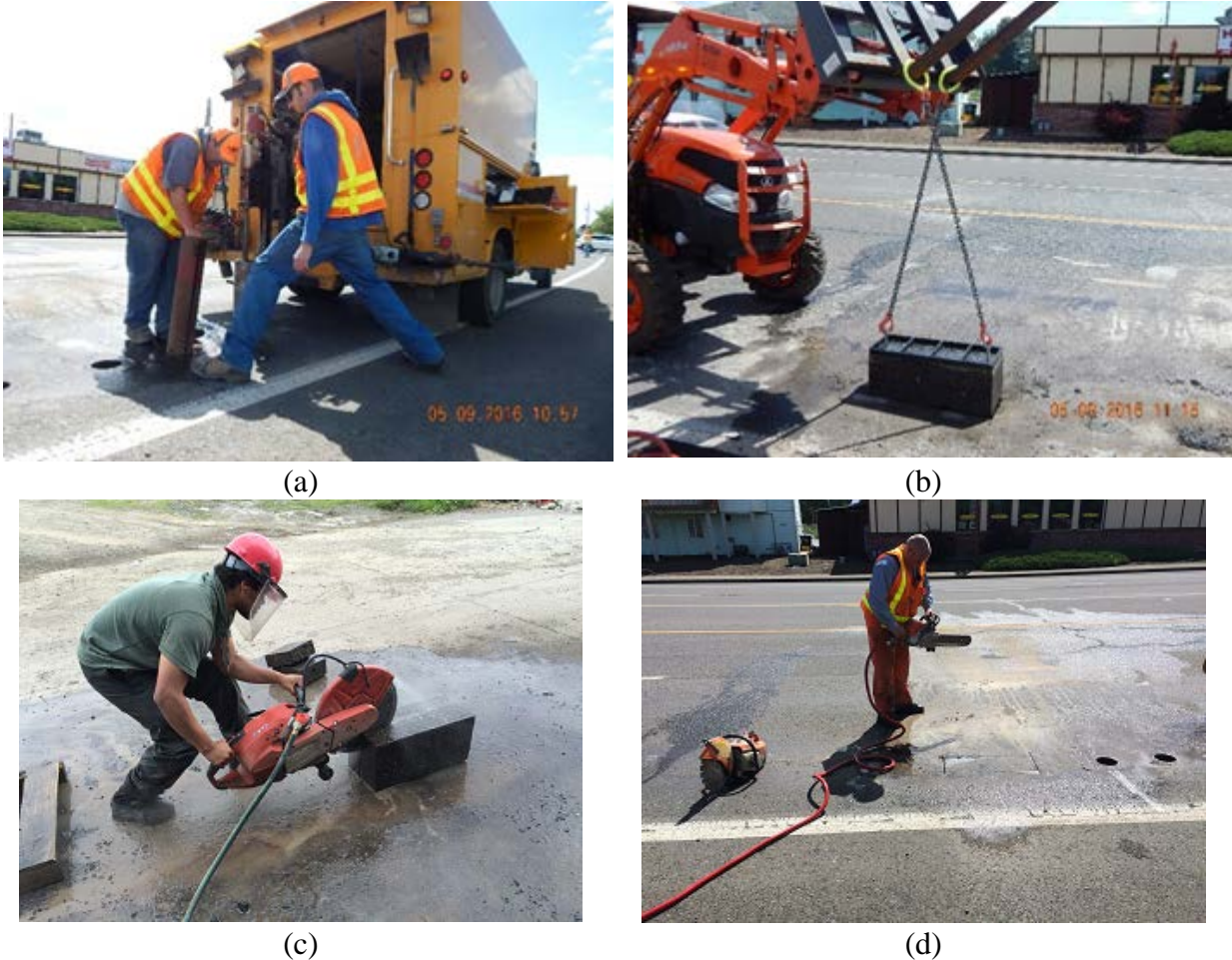
Figure 3.4: Field sampling (a) Cores for SCB and IDT tests (b) Slab samples for BBF test (c) Cutting field slabs to produce blocks that can fit the lab saw (d) Cutting field blocks.
