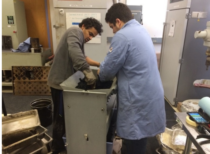
Figure 3.5: Mechanical Splitting of Asphalt Mixtures
