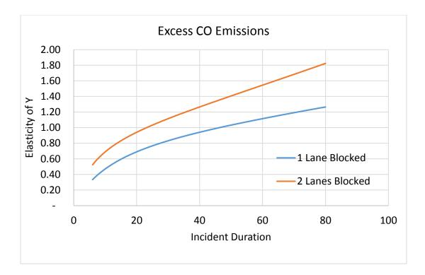
Figure 7-7. Elasticity of Excess CO Emissions with respect to incident duration
