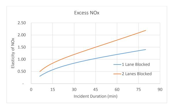
Figure 7-9. Elasticity of Excess NO<sub>x</sub> Emissions with respect to incident duration
