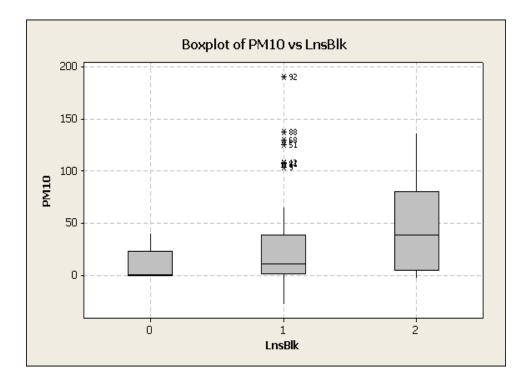
Figure 5-26. Box-plot: Excess PM<sub>10</sub> emissions (in Grams) vs. Number of Blocked lanes
