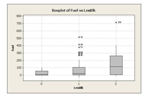
Figure 5-14. Box-plot: Excess Fuel Consumption (in gallons) Vs. Number of Lanes Blocked
