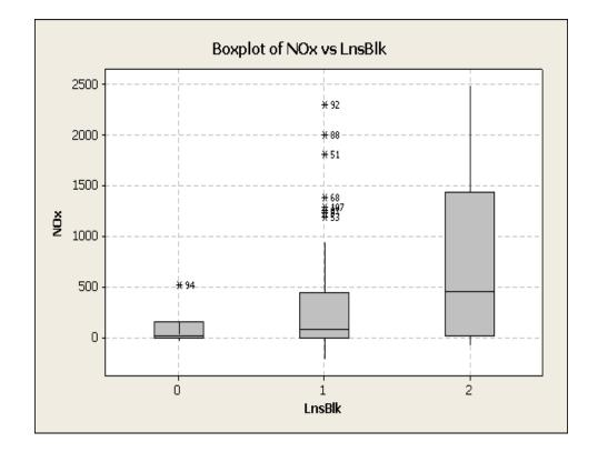
Figure 5-23. Box-plot: Excess NO<sub>x</sub> emissions (in Grams) vs. Number of Blocked lanes
