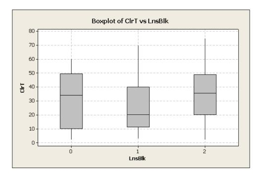
Figure 5-2. Box-plot: Incident Duration Vs. Number of Blocked Lanes
