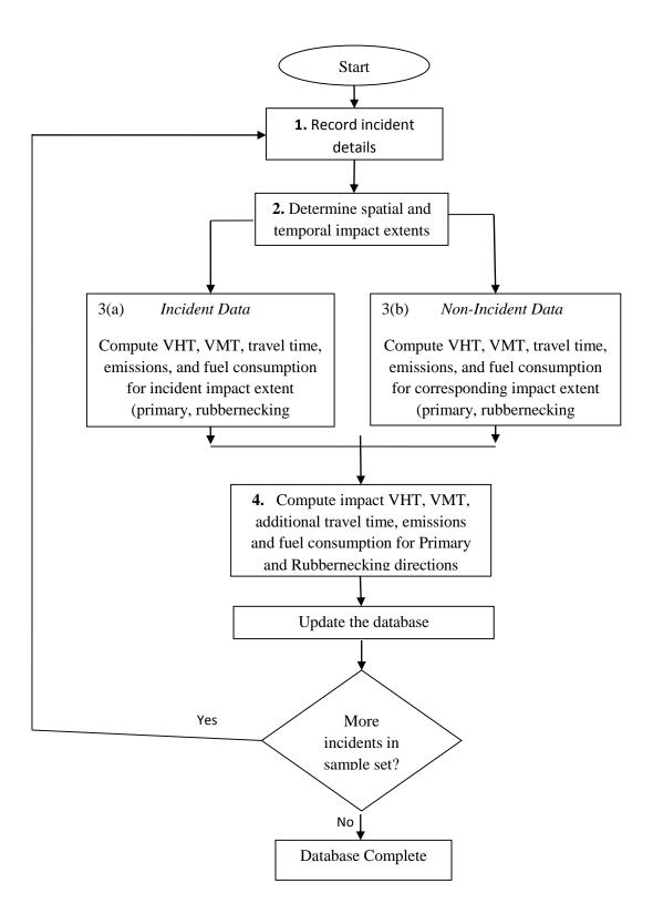
Figure 3-6. Flowchart for Generation of the Analysis Database
