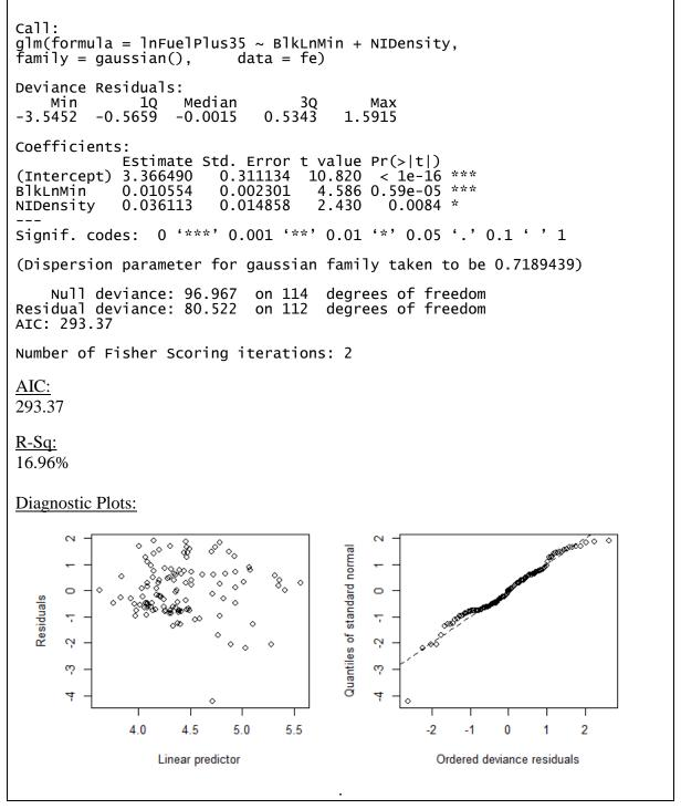
Figure 6-5: Best Model Results Excess Fuel Consumption (gallons) (Model Form: Gaussian Single-log GLM)
