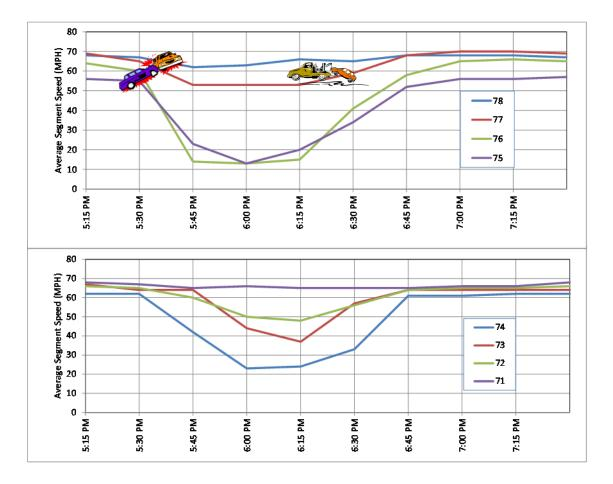
Figure 4-6. Speed-Segment Plot showing Spatial and Temporal extents of Sample Incident
