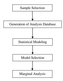
Figure 3-5. Flowchart for Modeling Incident Impacts on Travel Time, Emissions and Fuel Consumption
