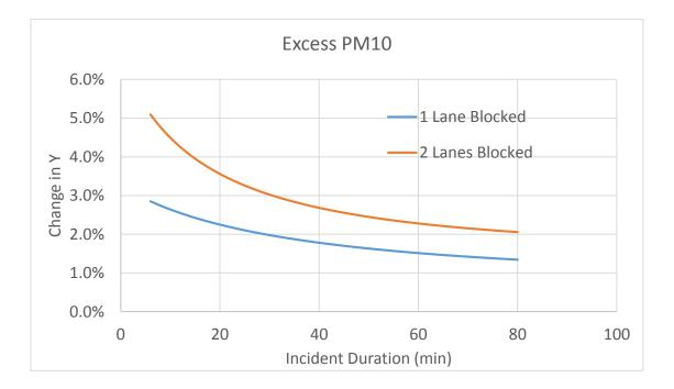
Figure 7-12. Percent Change in Excess PM<sub>10</sub> Emissions for 1 minute change in incident duration
