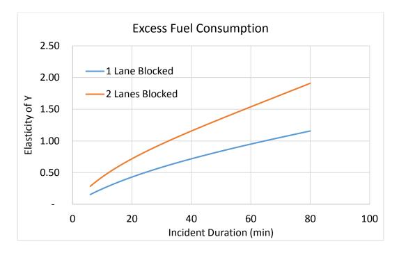
Figure 7-3. Elasticity for Lane-Minutes of Blockage in Excess Fuel Consumption
