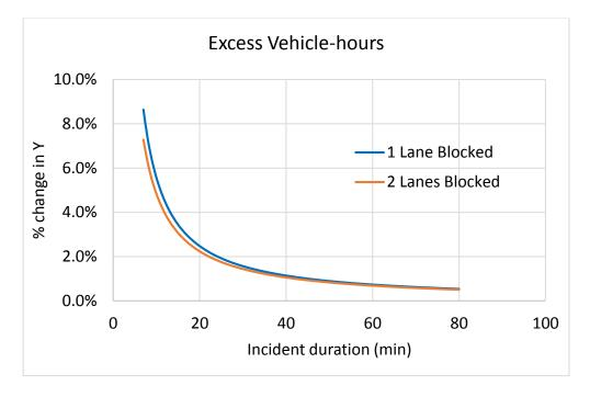
Figure 7-2. Percent Change in Excess VHT for unit change in Incident Duration
