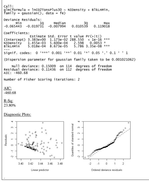
Figure 6-6. Best Model: Excess CO<sub>2</sub> Emissions (Tons) (Model Form: Gaussian Single-Log GLM)
