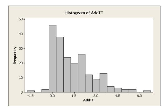
Figure 5-3. Histogram: Additional Travel Time per vehicle (Mean value = 1.32; Median = 1.05 minutes/vehicle)
