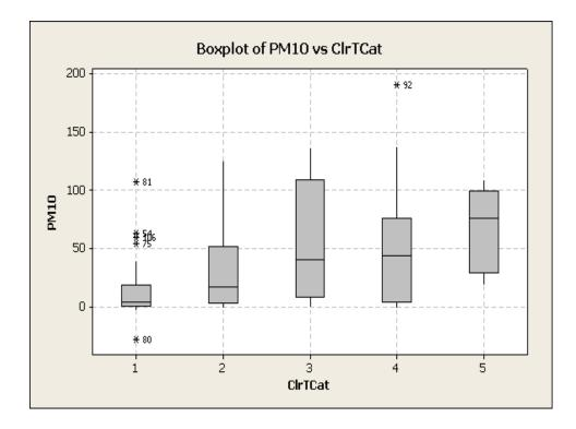
Figure 5-27. Box-plot: Excess PM<sub>10</sub> emissions (in Grams) vs. Incident Duration
