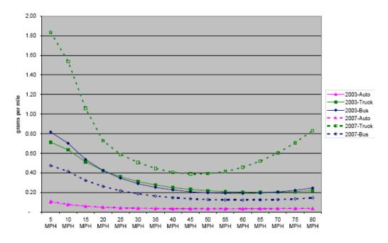
Figure 3-4. PM<sub>10</sub> Emissions versus Speed
