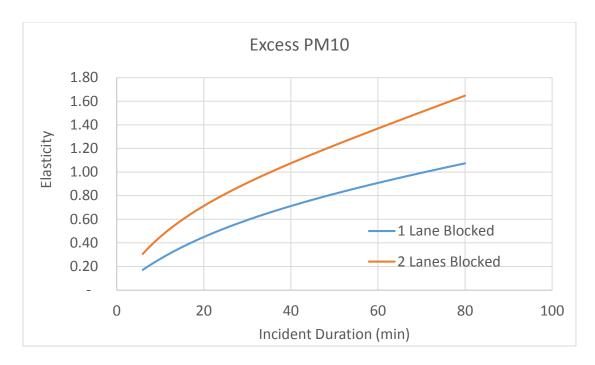
Figure 7-11. Elasticity for Excess PM10 emissions with respect to Incident Duration
