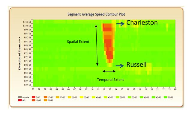
Figure 3-7. Speed Plot for Sample Incident
