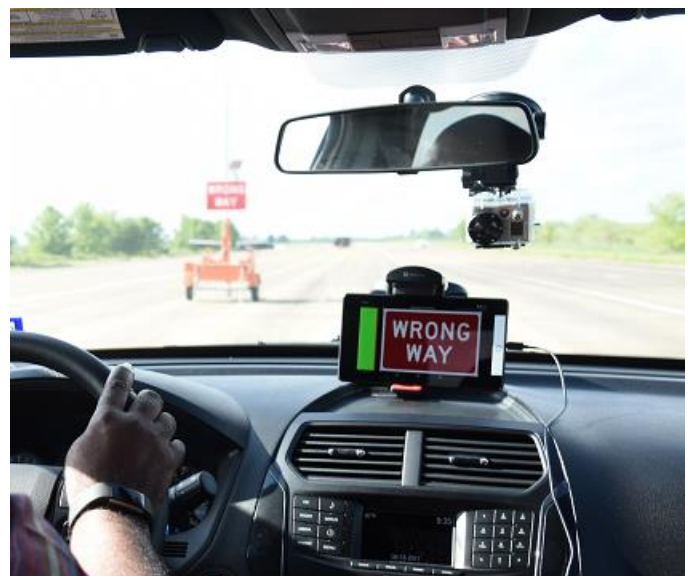
Figure 2. In-Vehicle Warning Message for the Wrong-Way Vehicle Display.
