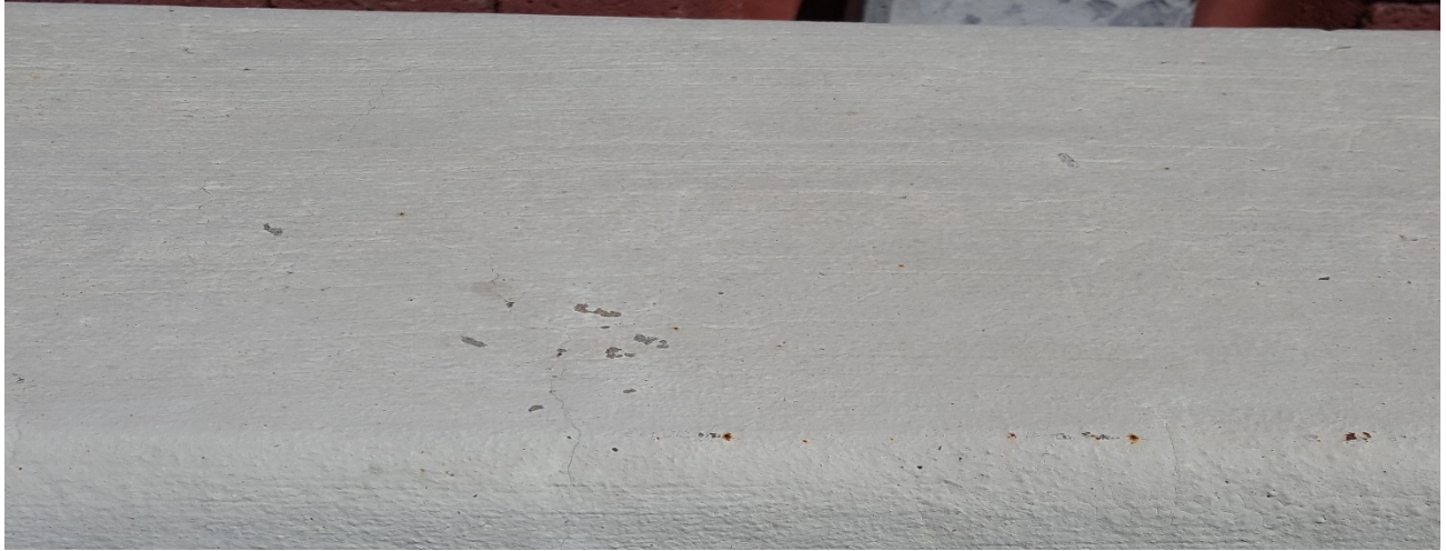
Klaas Coatings – (B), (W) Delamination, but much less compared to (UB), (W)
