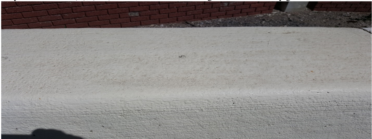
ChemMaster (B), (LM) No delamination. Coating intact. Looks very good.
