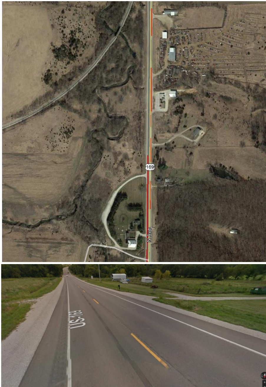
Figure 5. Rumble strip installation with gaps at driveways
