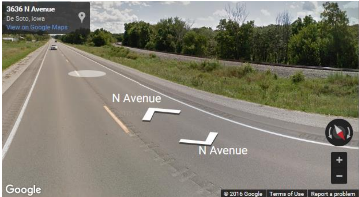
Figure 2. Right continuous with left intermittent
