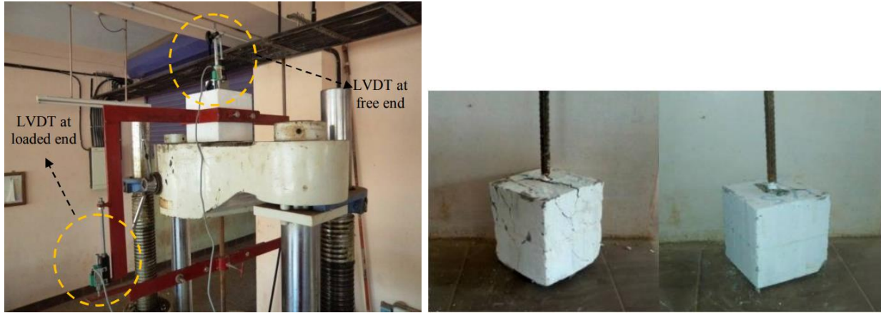
Figure A.37 Test Setup (left) and the Failed Pullout Specimens (right) (Source: Deepthi and Sabeena, 2016)
