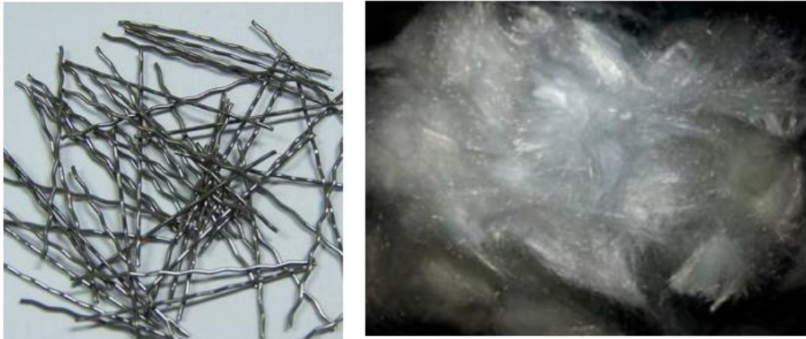
Figure A.35 Steel Crimped Fibers ( left ) and Recron 3S Fibers ( right ) (Deepthi and Sabeena, 2016)
