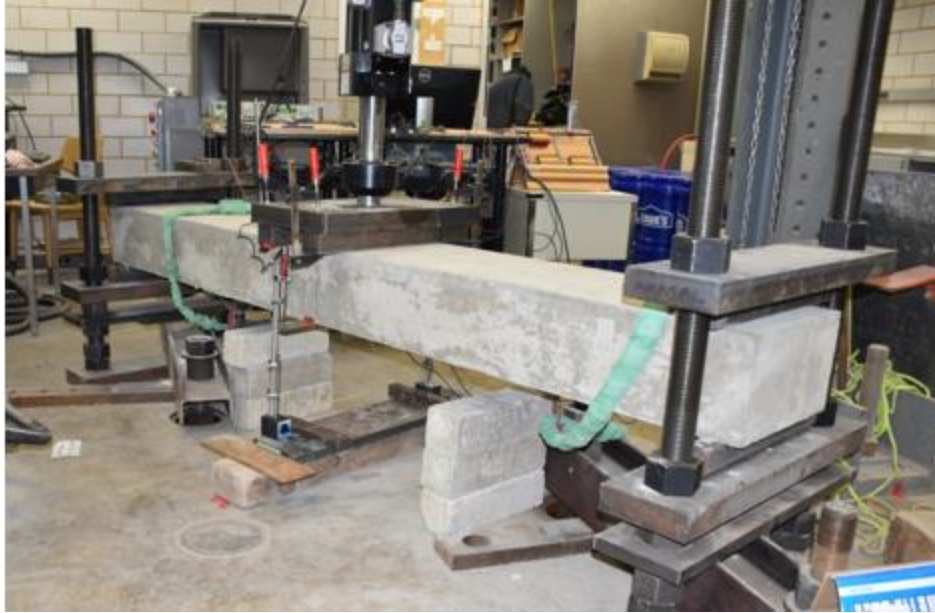
Figure F.63 Fatigue Loading on a Slab to Monitor Crack Widening
