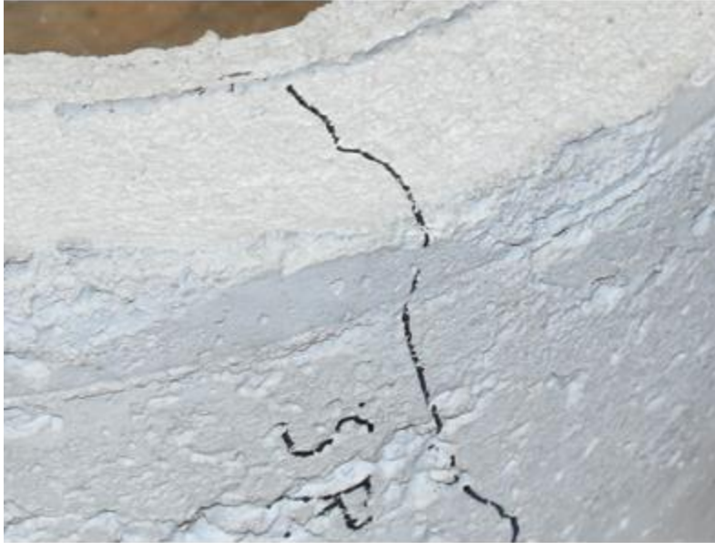
Figure E.29 Cracking in SRA Specimen at 14 to 15 Days
