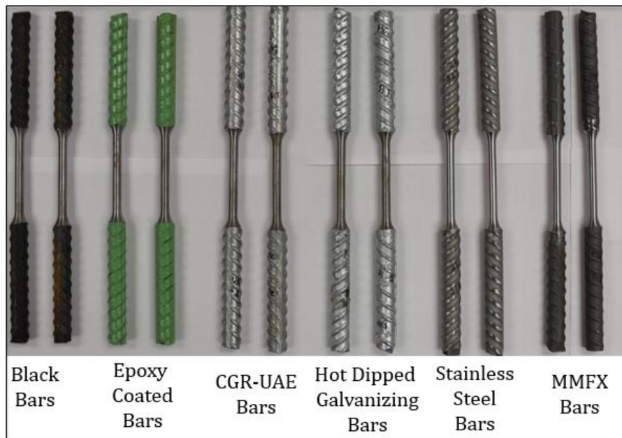
Figure F.1 Various Reinforcement Bars Machined at the Center for Tensile Strength Testing
