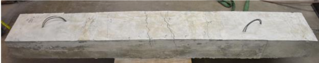
Figure F.52 Failed 13" \times 8" Slab Specimen Showing Crack Pattern
