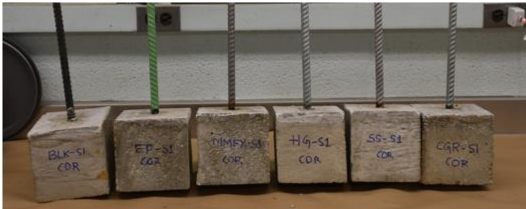
Figure D.24 Tested Pullout Specimens with Fibers and Corroded
