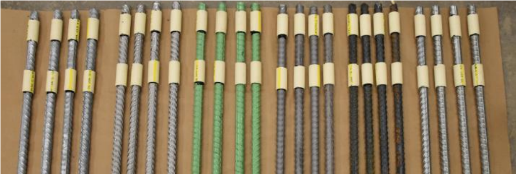
Figure D.16 Bond Breaker Applied on Bars
