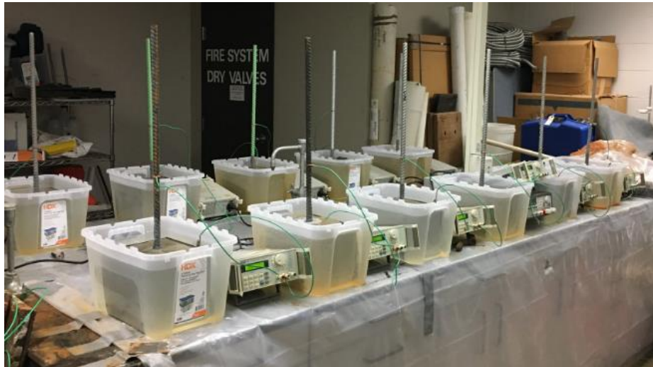
Figure D.21 Test Setup of Pullout Specimens Subjected to Accelerated Corrosion
