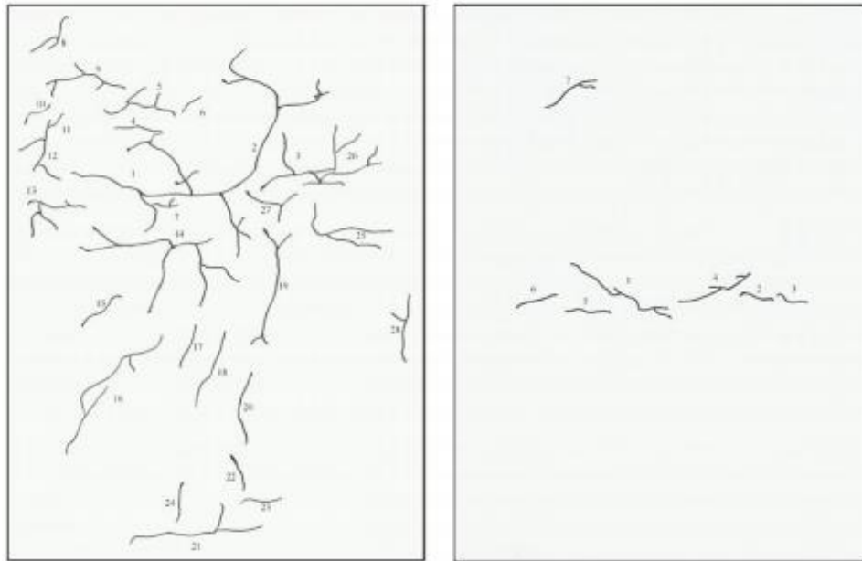
Figure A.8 Typical Plot of Crack Patterns of Test Slabs Without Fibers ( left ) and With 0.3 \text{ kg/m}^3 ( 0.5 \text{ lbs/yd}^3 ) Monofilament Fibers ( right ) (Ramakrishnan, Zellers and Patnaik et al., 2007)
