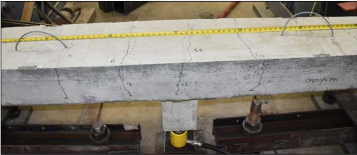
Figure G.21 Cracks in Specimen with a Pin Connection
