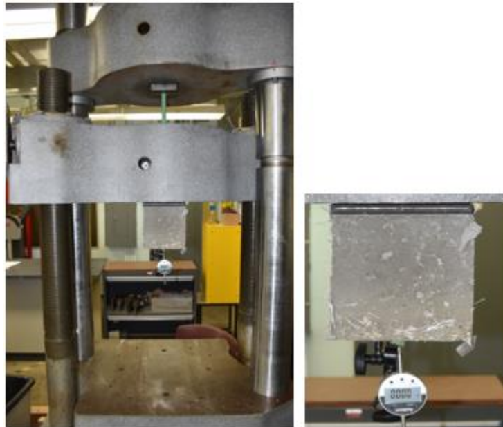
Figure D.23 Test Setup for Pullout Specimens (left) and Dial Gage Setup (Right)
