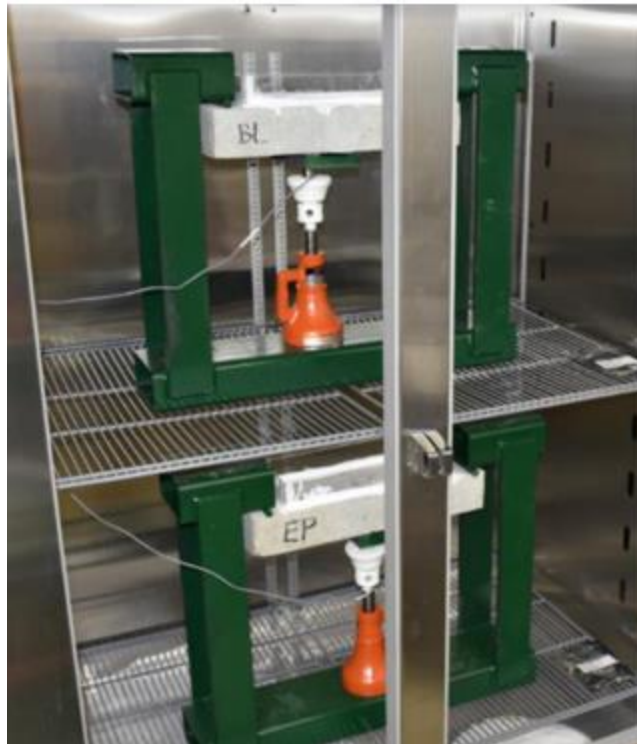
Figure E.41 Loaded Freeze-Thaw Test Setup inside the Chamber
