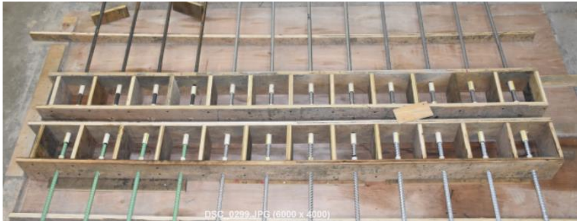
Figure D.17 Formwork of Pullout Specimens
