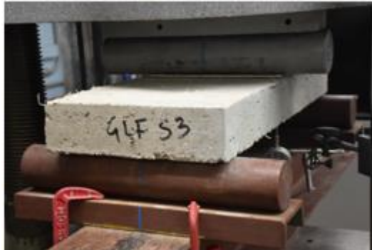
Figure D.9 Flexure Test on Pristine Slab
