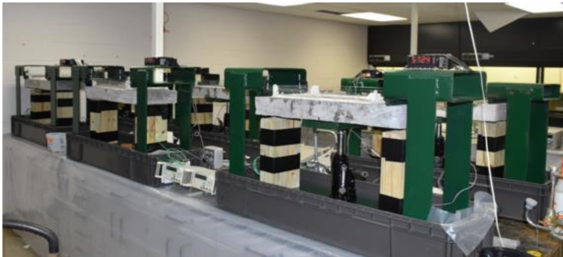
Figure D.8 Typical Setup of Specimens Undergoing Accelerated Corrosion
