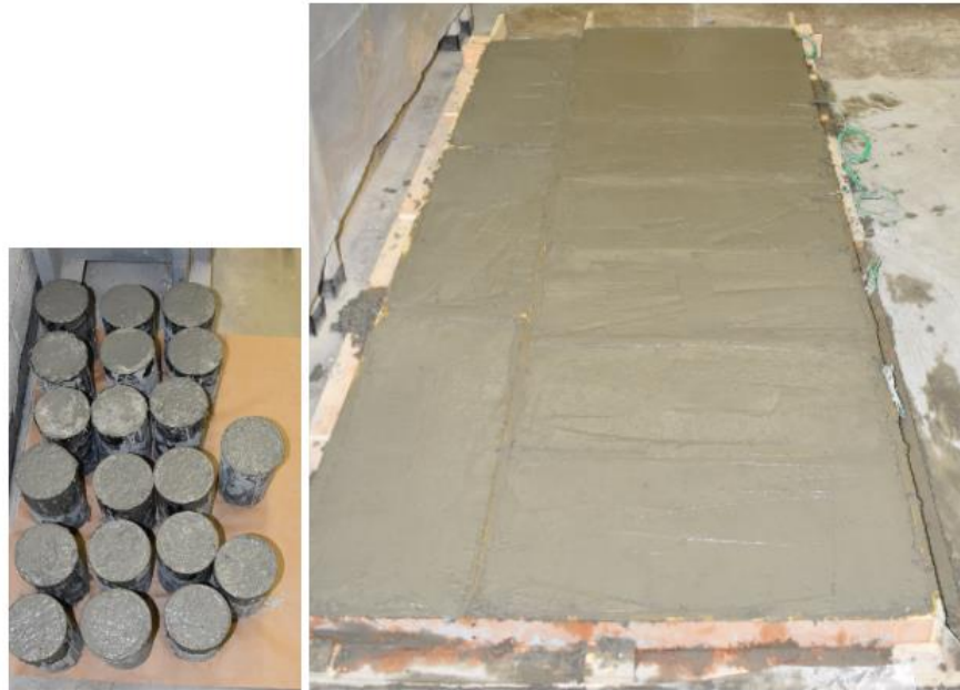
Figure D.4 Casting of Test Slabs for Corrosion Testing
