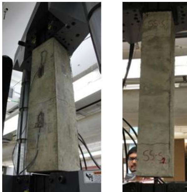
Figure F.9 Testing of Prisms in Trial I (Left) and Trial II (Right)
