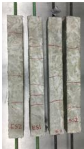
Figure F.14 Cracks Formed on Specimens during Testing in Trial III
