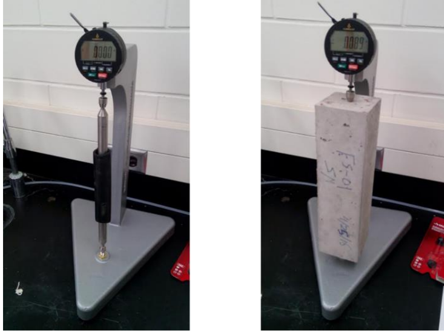
Figure E.17 Measurement of Free Shrinkage using ASTM C490
