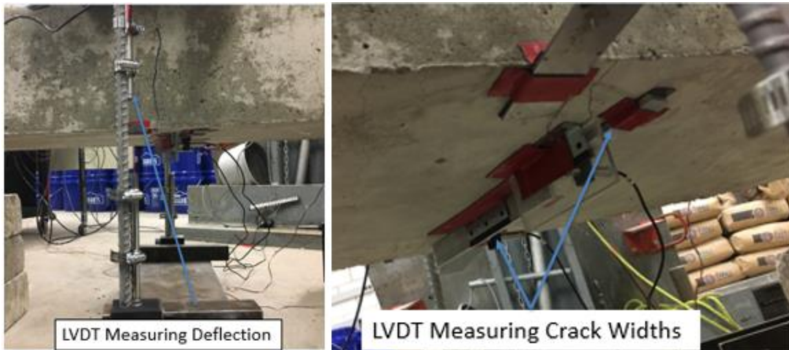
Figure F.64 Slab Showing LVDTs to Measure Deflection ( Left ) and Crack Width ( Right )
