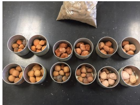
Figure 2-2 LWA made from dredged material taken from the Harbor of Cleveland
