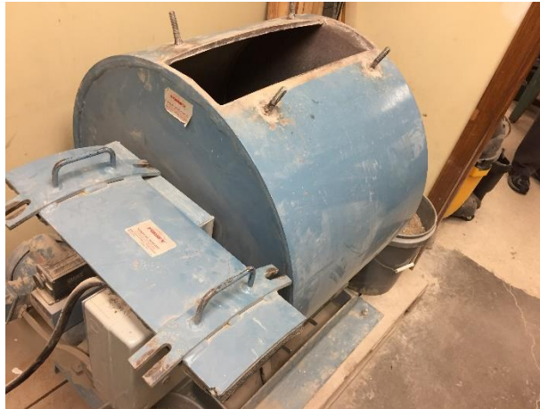
Figure 3-5 LA Abrasion Machine
