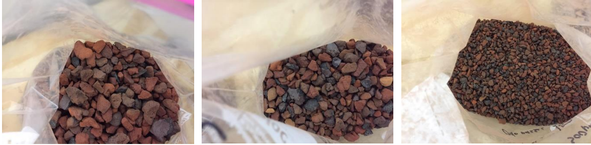
(a) Coarse (max. 25 mm, 1.0 in.) (b) Coarse (max. 19 mm, 0.75") (c) Fine (max. 4.75 mm, 0.187")
