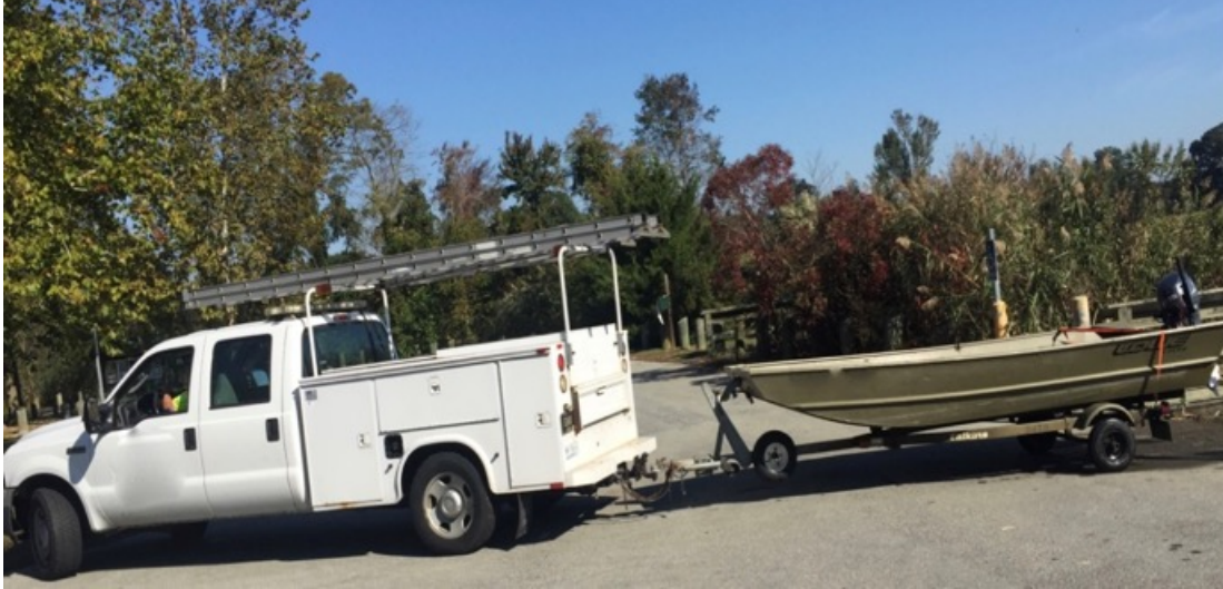
Figure 3.4: Bridge inspection motor boat attached to the inspection truck
