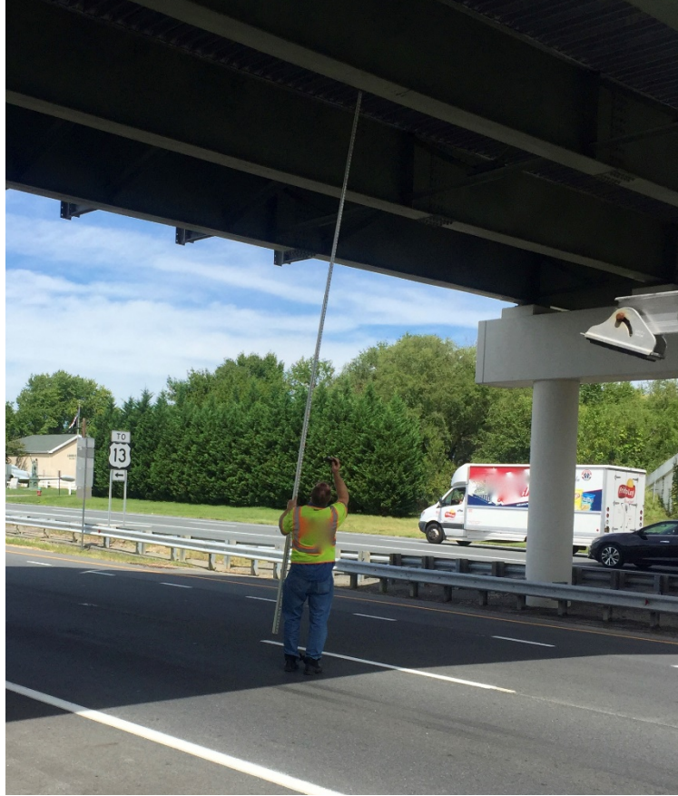
Figure D-5: Checking clearance of the bridge
