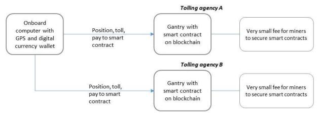
Figure 16. Using Smart Contracts and Onboard Computer to Pay Tolls.
