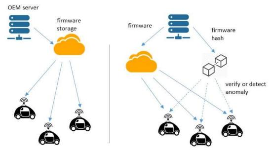
Figure 13. Using Blockchain to Verify Firmware Update over the Air.
