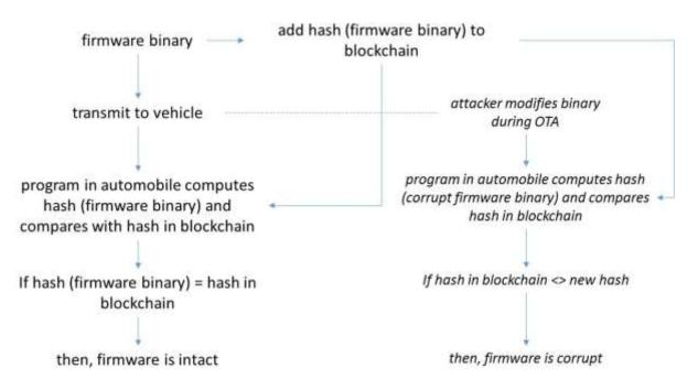
Figure 14. Using Firmware Hash in Blockchain to Verify Updates.
