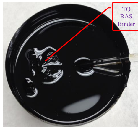
Figure 3-7. TO shingle binder and virgin binder blended at 163°C
