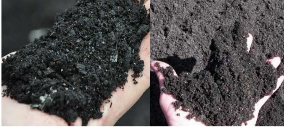
Figure 2-2 Normal grind RAS (left) and finer grind RAS (right)
