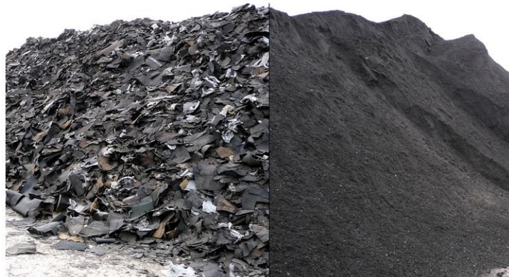
Figure 2-1. RAS stockpile before (left) and after (right) grinding
