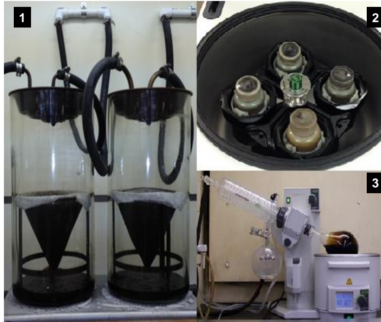
Figure 3-2. Asphalt binder extraction and recovery
