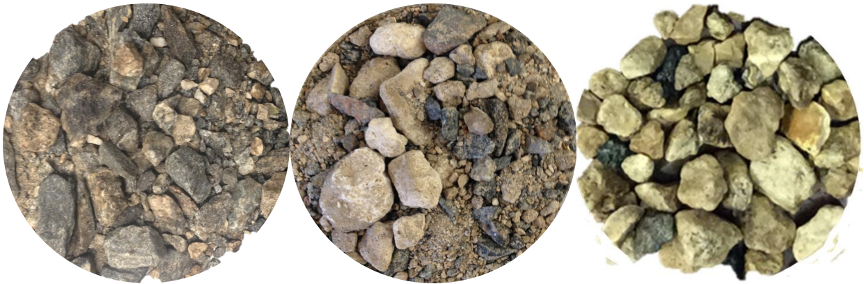
Figure 3-10. Aggregate components of ATL RAP (left), ACO RAP (middle) and WHI RAP (right)
