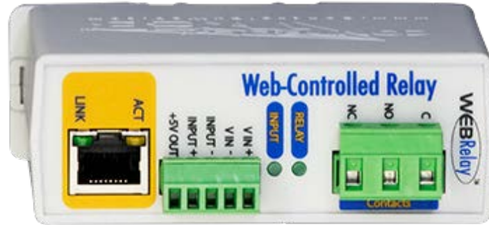
Figure 32. WebRelay Hardware Device.
