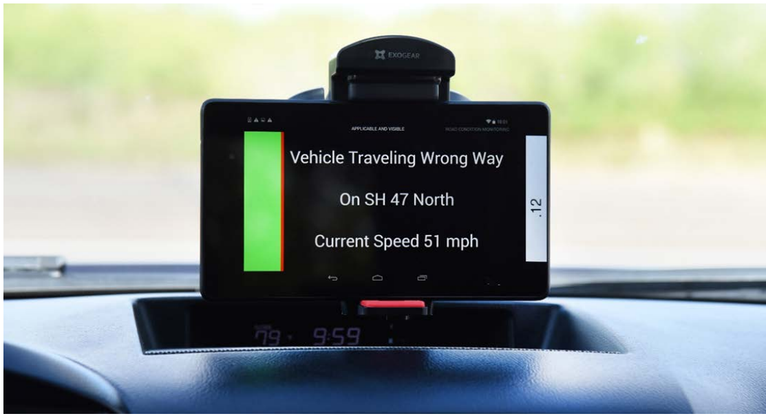
Figure 10. Information Displayed to Connected Law Enforcement Vehicle.
