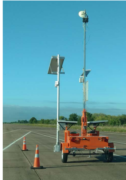
b) Trailer with a Pole-Mounted RSU and Communication Antenna (Foreground) and TAPCO Detectors (Background).
