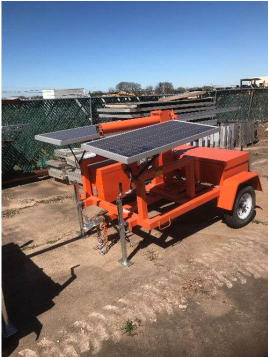
a) Trailer for Powering and Temporarily Mounting an RSU.
