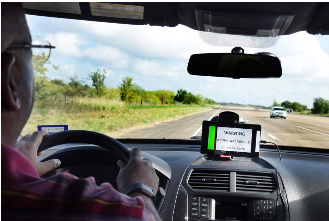
Figure 9. Warning Message That Appears on Right-Way Driving Vehicle's Tablet.
