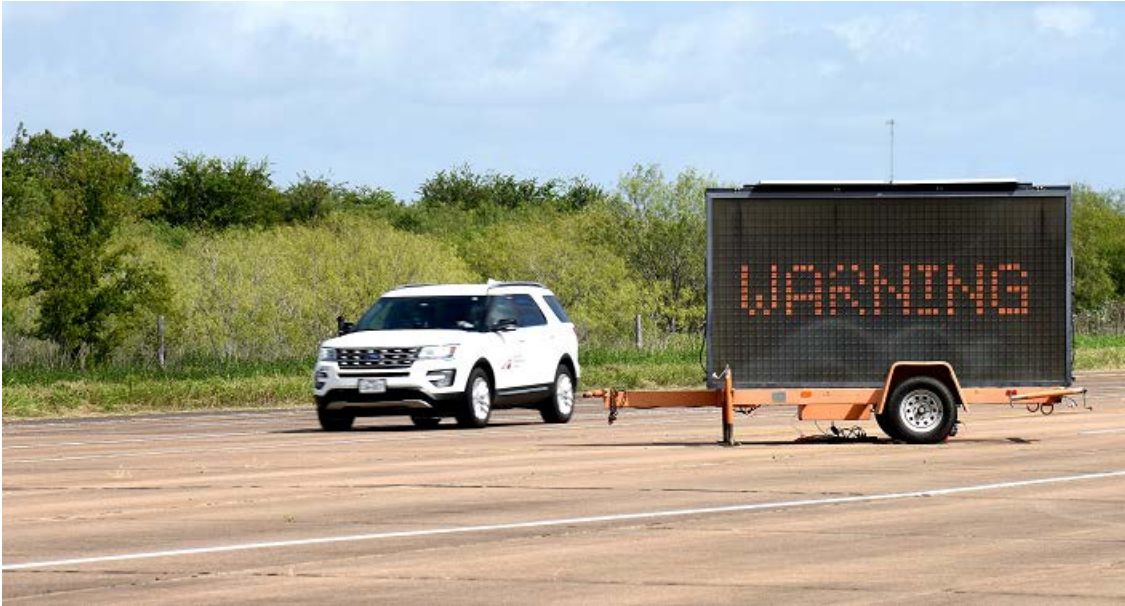
Figure 4. A PCMS Displaying a Warning about the Existence of a Wrong-Way Driving Vehicle.
