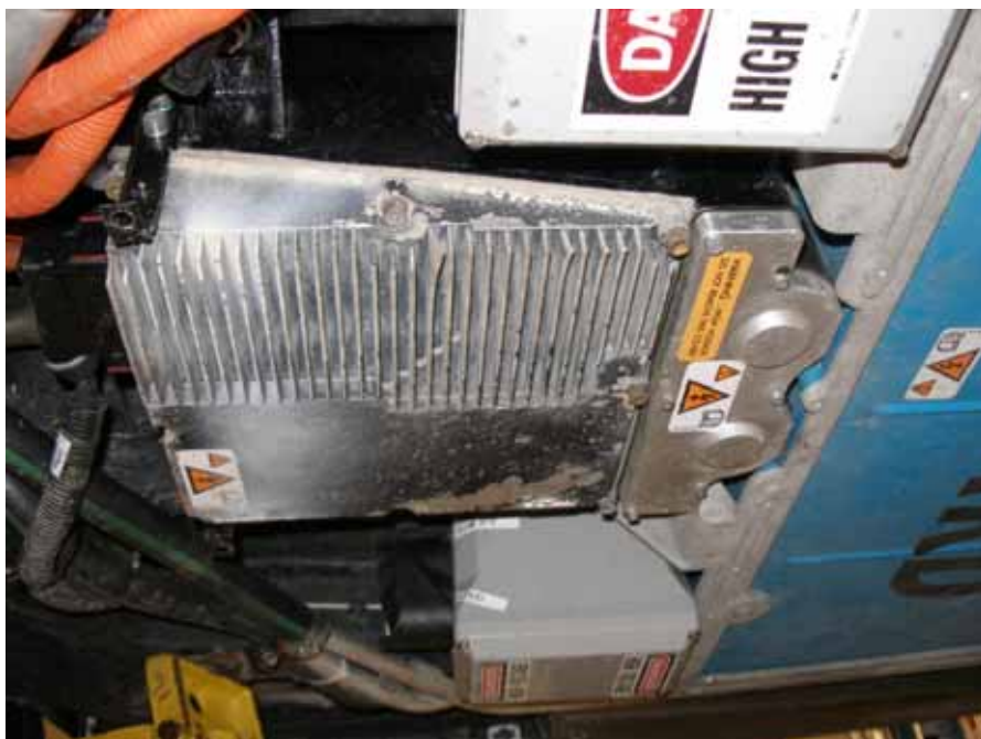
Figure 3. Ford Focus fuel cell (blue box) and electronic/disconnects enclosure.
