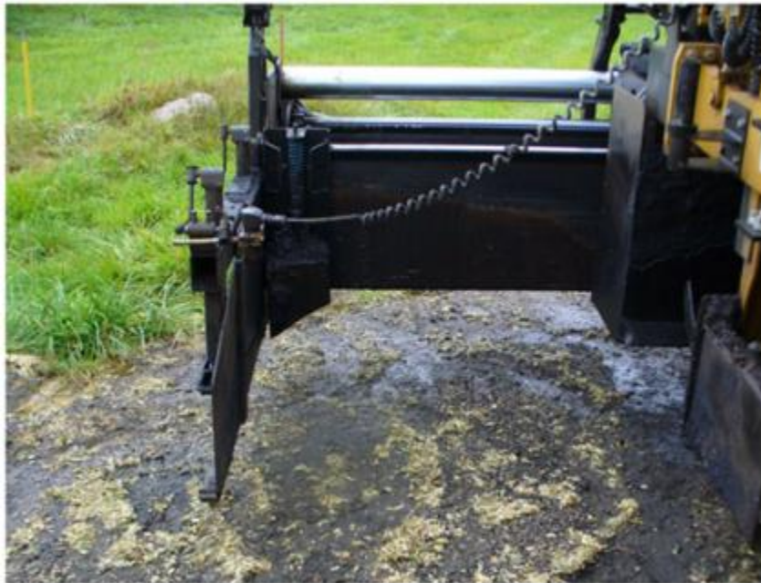
Figure 14. Advant-Edger™ mounted on a paver. Unit is designed to automatically adjust to shoulder elevation changes (driveways and intersections).
