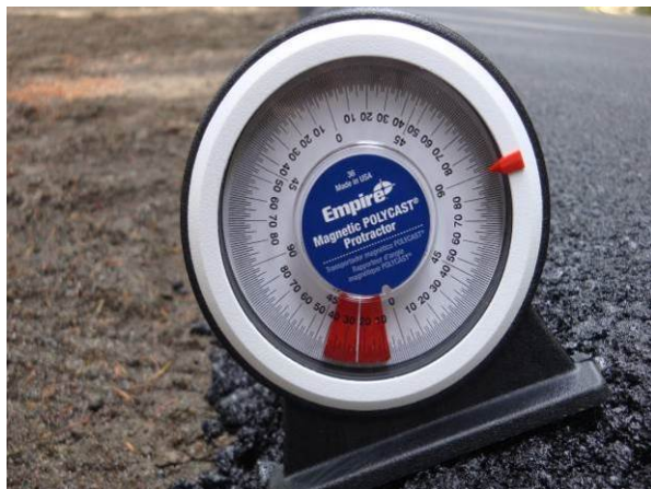
Figure 57. Close-up of slope indicator.
