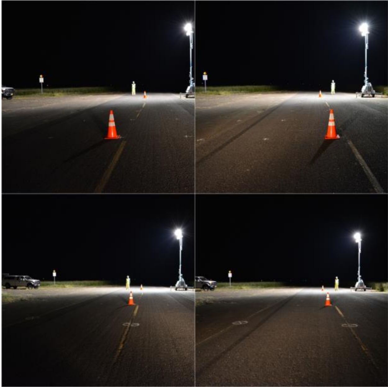
Figure 7.12: Comparison of Worker Visibility at Different Positions relative to Light Tower
