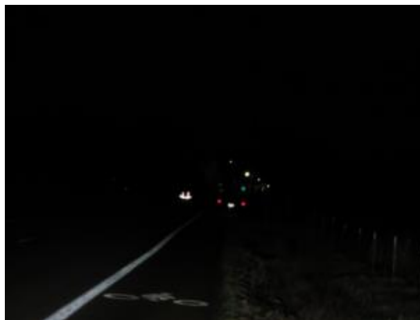
Figure 2.10: Class 3 High Visibility Vests as Seen at Night from 500 feet
