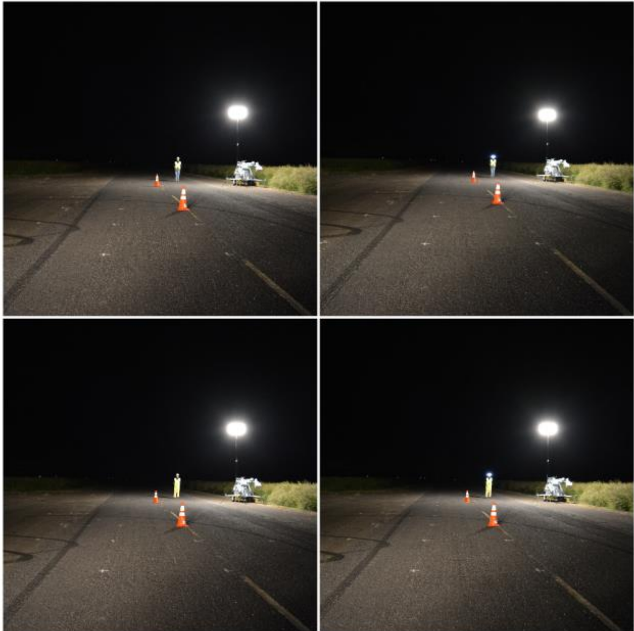
Figure 7.5: High Visibility Apparel under Balloon Light from 100 feet Away
