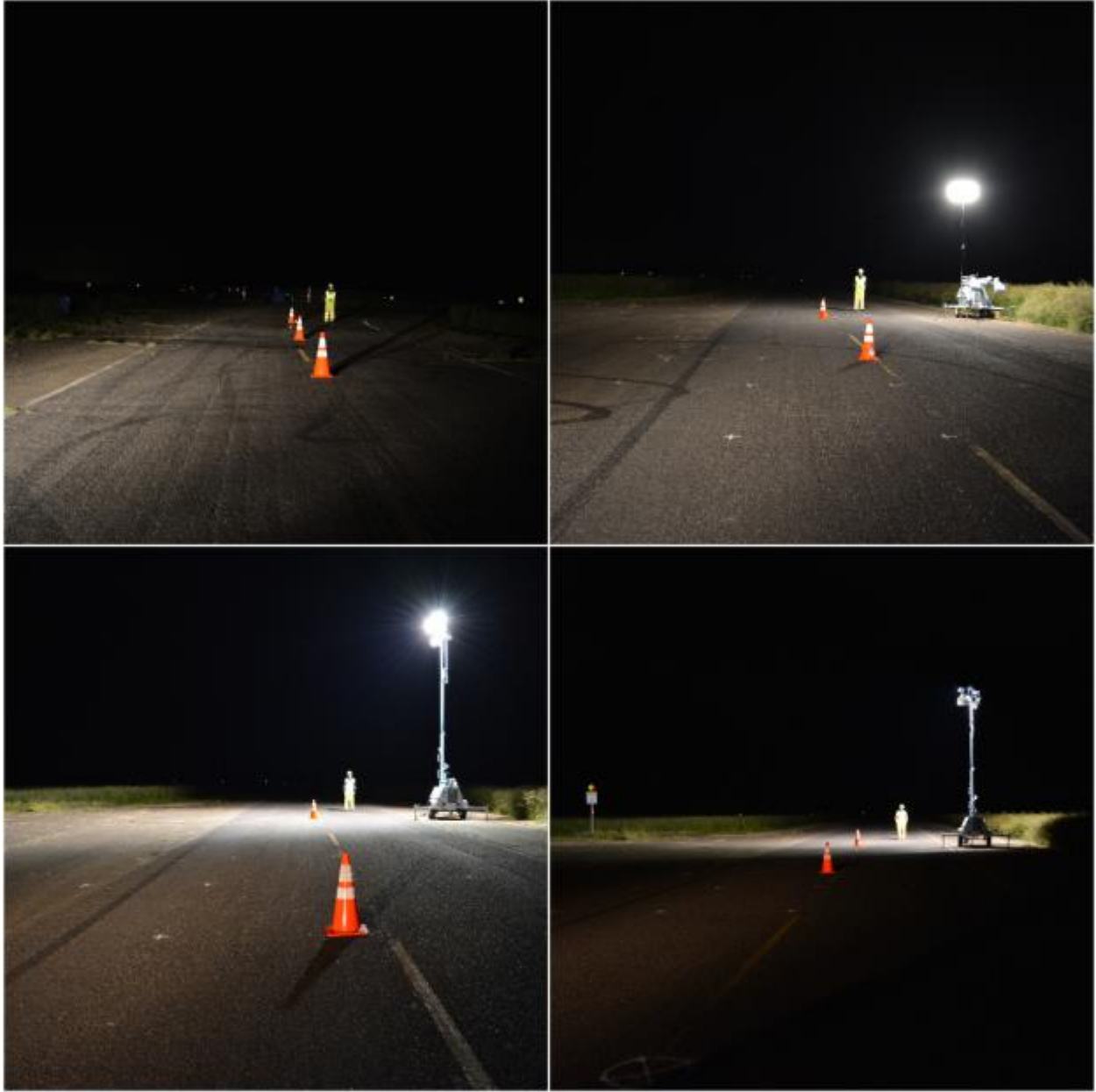
Figure 7.15: Visibility of Worker under Different Lighting Equipment from 100 feet Away
