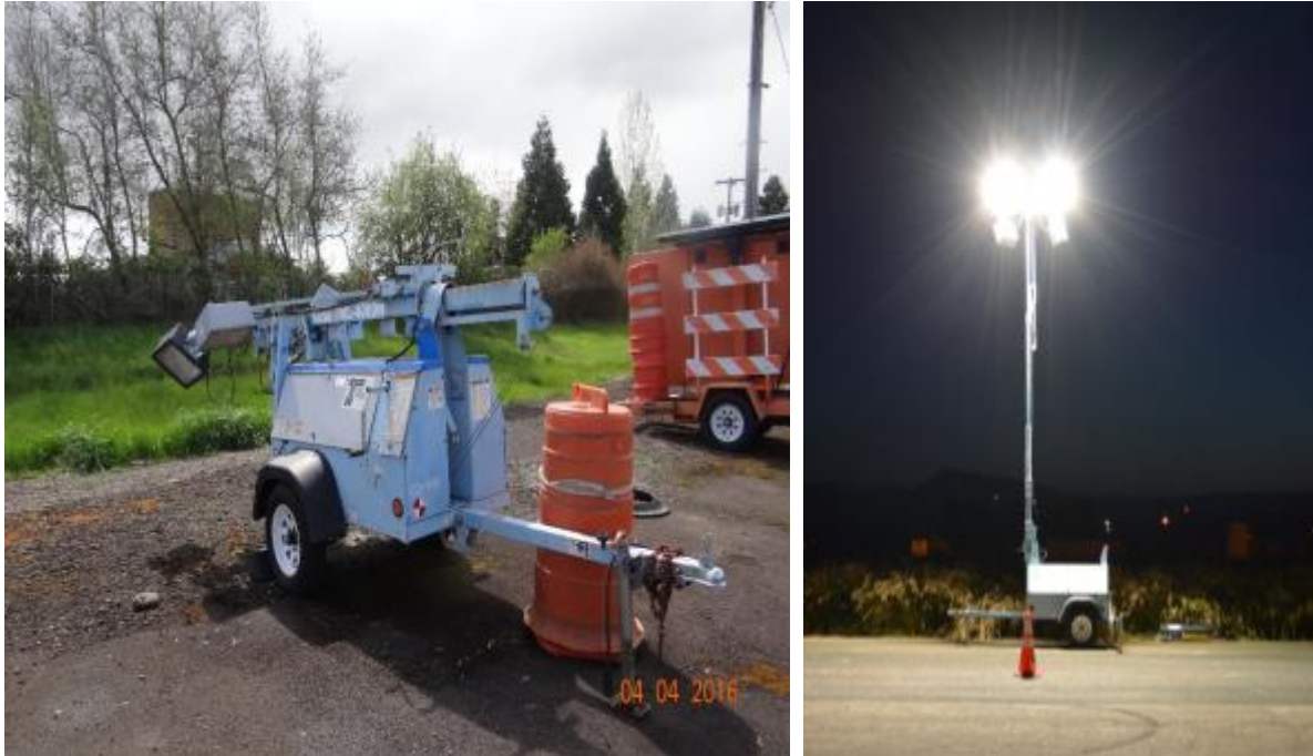
Figure 2.1: Portable Trailer-mounted Light Tower with Mast Lowered and Mast Raised
