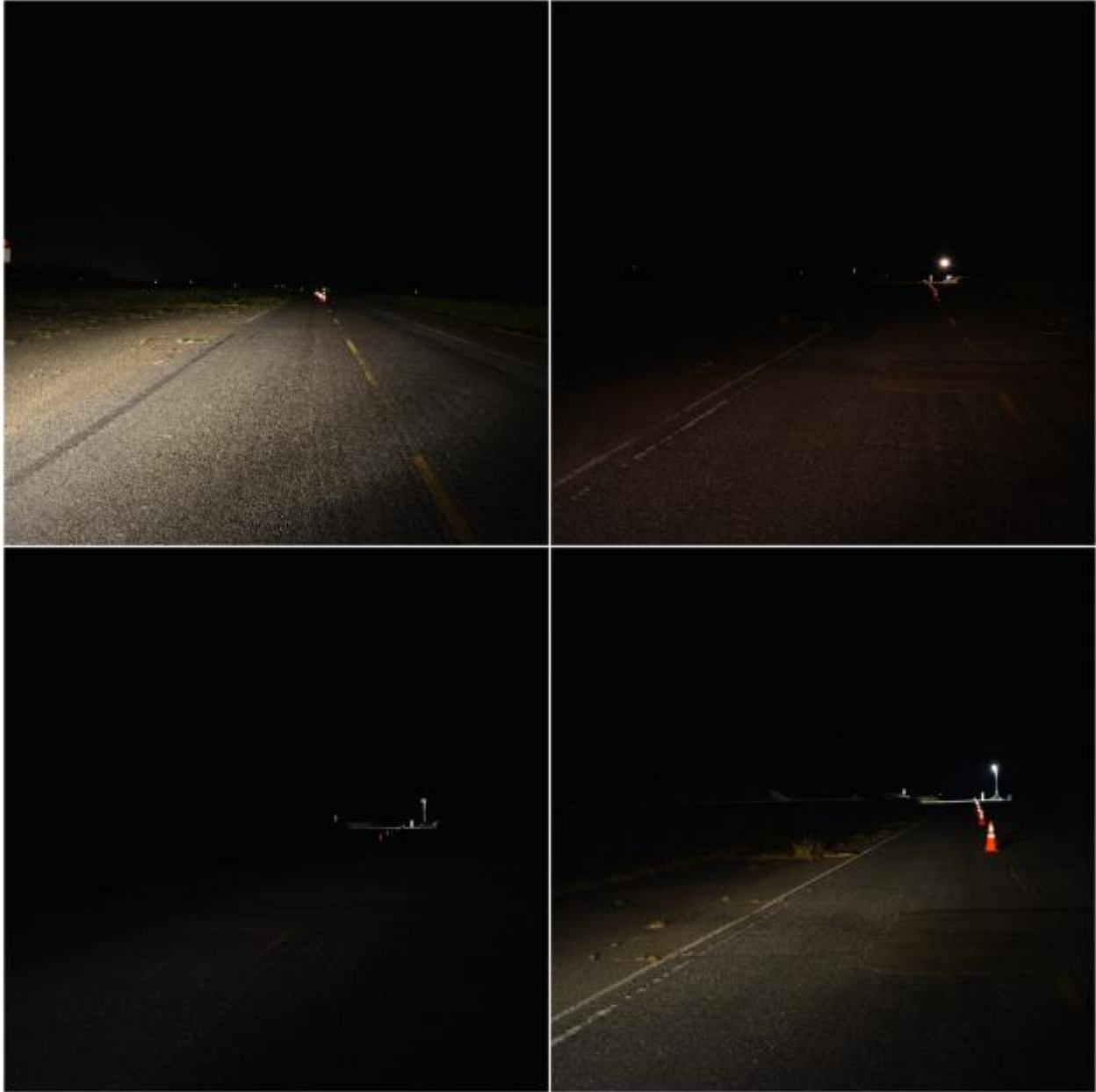
Figure 7.16: Visibility of Worker under Different Lighting Equipment from 500 feet Away
