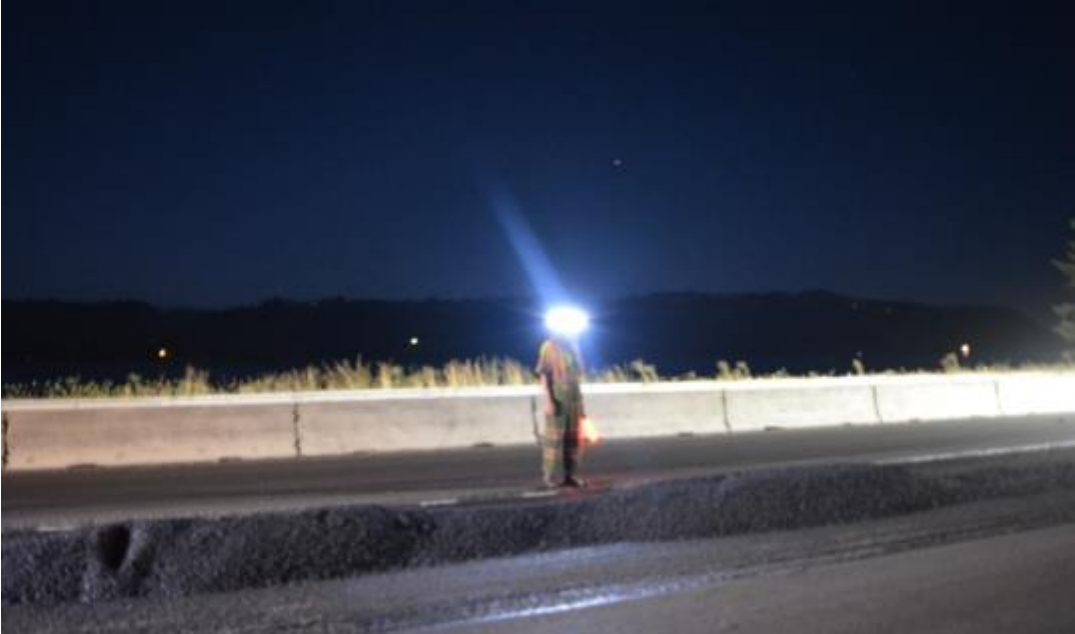
Figure 9.38: Visibility of Worker Wearing Dirty Reflective Garments and Halo Light
