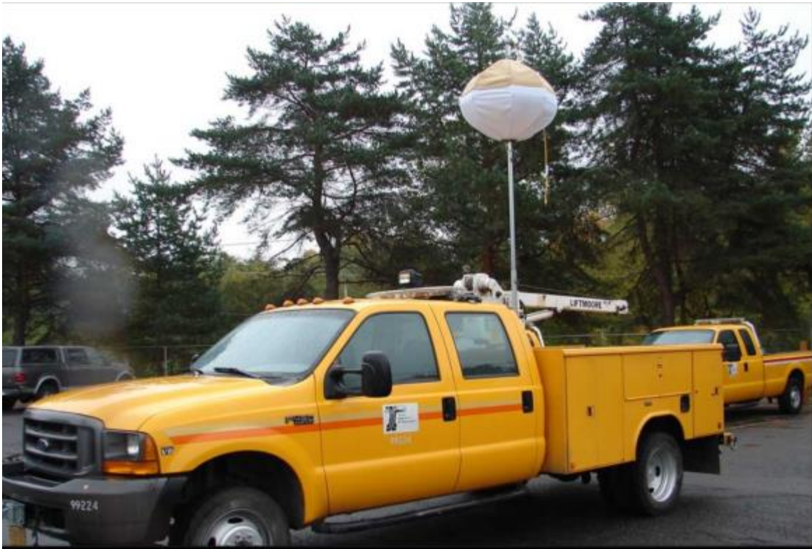
Figure 5.11: Example of Balloon Light Mounting for Density Technician Truck
