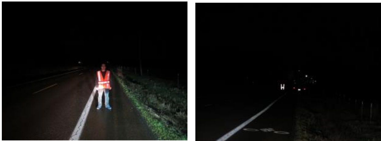
Figure 2.8: Class 2 High Visibility Vests as Seen at Night from 20 feet (left) and 500 feet (right)
