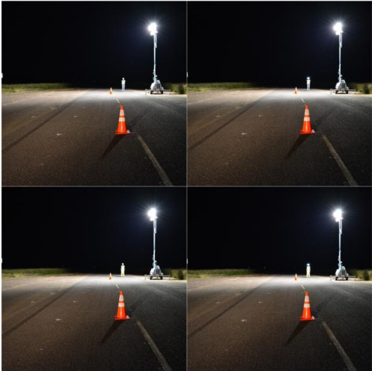
Figure 7.11: Comparison of High Visibility Apparel under Light Tower from 100 feet Away
