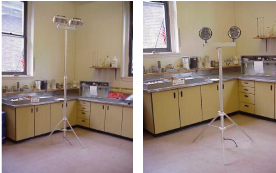
Figure 2.4: Tripod-Mounted Floodlights (left) and Spotlights (right) (Gambatese, 2005)
