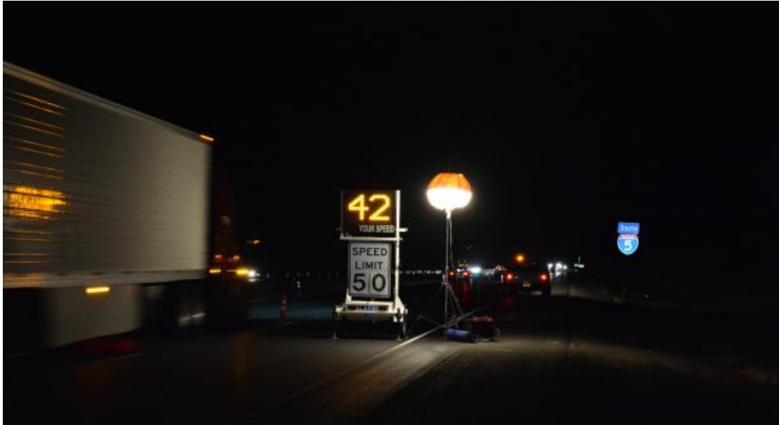
Figure 8.13: Radar Speed Trailer with Balloon Light, I-5 Medford to Ashland (Case Study #2)
