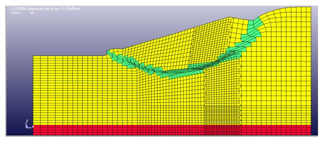
(B): Unmitigated failure of a 2:1 slope embankment
