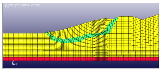
(A): Unmitigated failure of a 3:1 slope embankment
