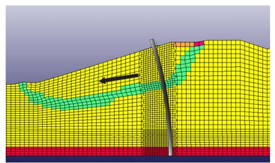
Figure 18: Deformed pile in 3:1 slope with deep failure
