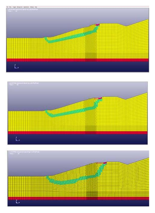
Figure 1: Embankments with 3:1 slope and varying depths of the failure zone
