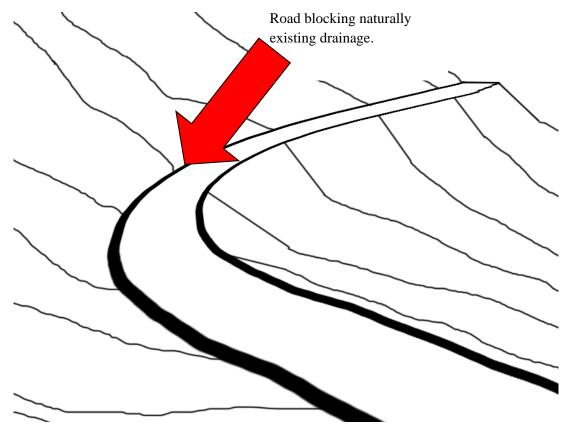
Figure 3. Naturally existing drainage blocked by road.
