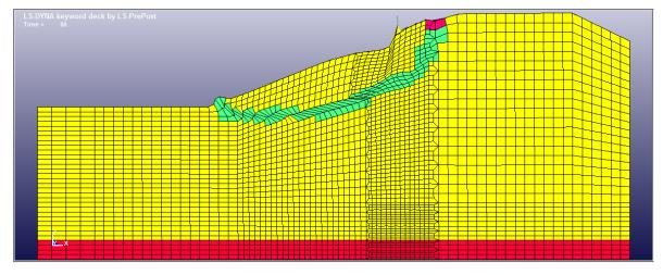
(C): Mitigation based on HP 18x204 driven piles spaced at 5 ft.
