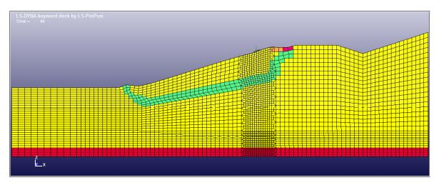
(B): Mitigation based on HP 14x102 driven piles spaced at 5 ft.
