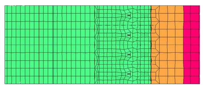
Figure 19: Soil flow between driven piles
