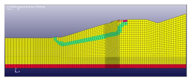
(C): Mitigation based on HP 18x204 driven piles spaced at 5 ft.
