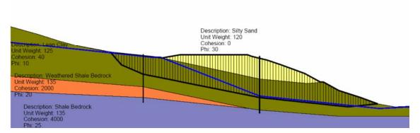
Figure 5: Soil stratification of the Muddy Pass Slide
