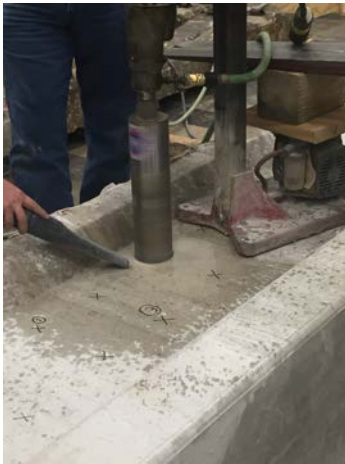
(a) Drilling cylinder from web
