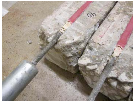
(b) Scaling/spalling at specimen ends
