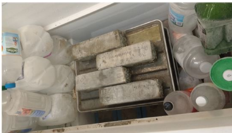
Figure 3.3. Specimens in freezer during freeze cycle.
