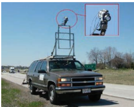
Figure A.3 Infrared thermography camera mounted on vehicle. (Photograph courtesy of Infrasense, Inc. (Maser et al., 2012).)
