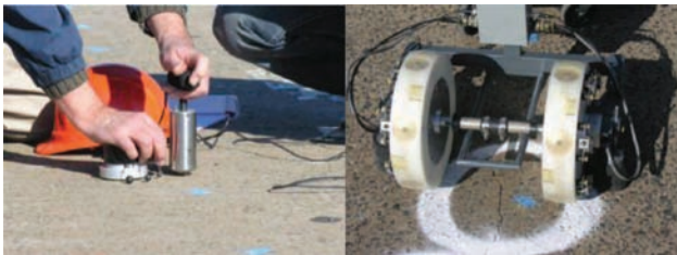
Figure A.10 Handheld impact echo in use (left). Rolling impact echo system (right). (Photographs Courtesy of Gucunski et al., 2013).
