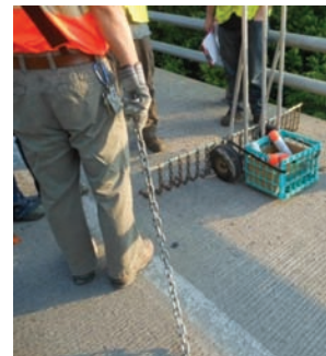
Figure A.2 Chain drag system used by INDOT.
