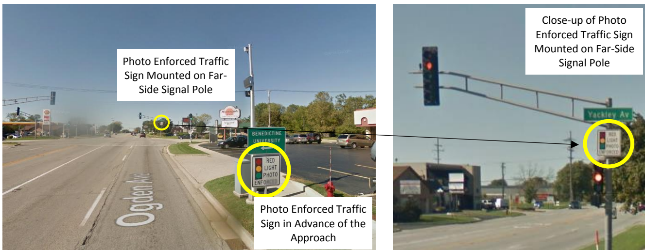
Figure 3.3 Photo-enforced sign placement at a sample test intersection.
