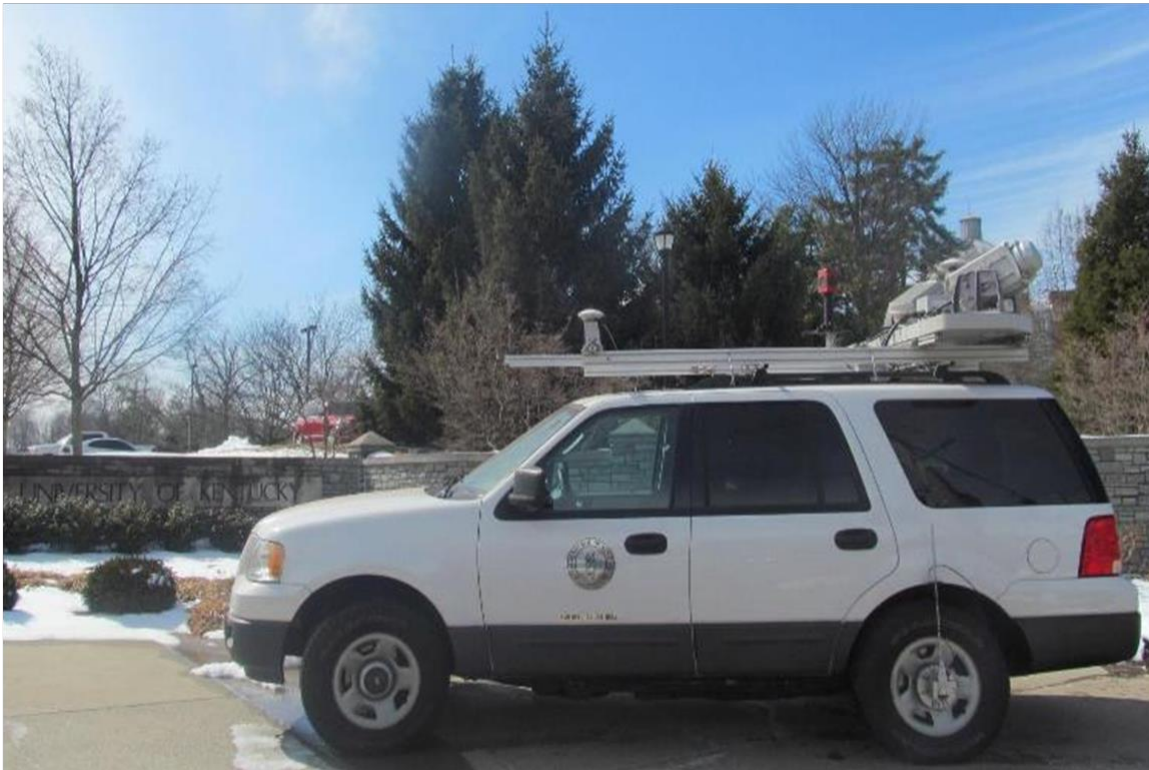
Figure 1 Lynx V200 mobile mapping system from Teledyne Optech
