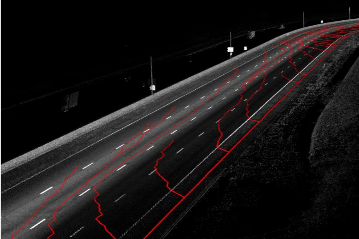
Figure 8 Water flow paths on I-75, Kenton County, Kentucky
