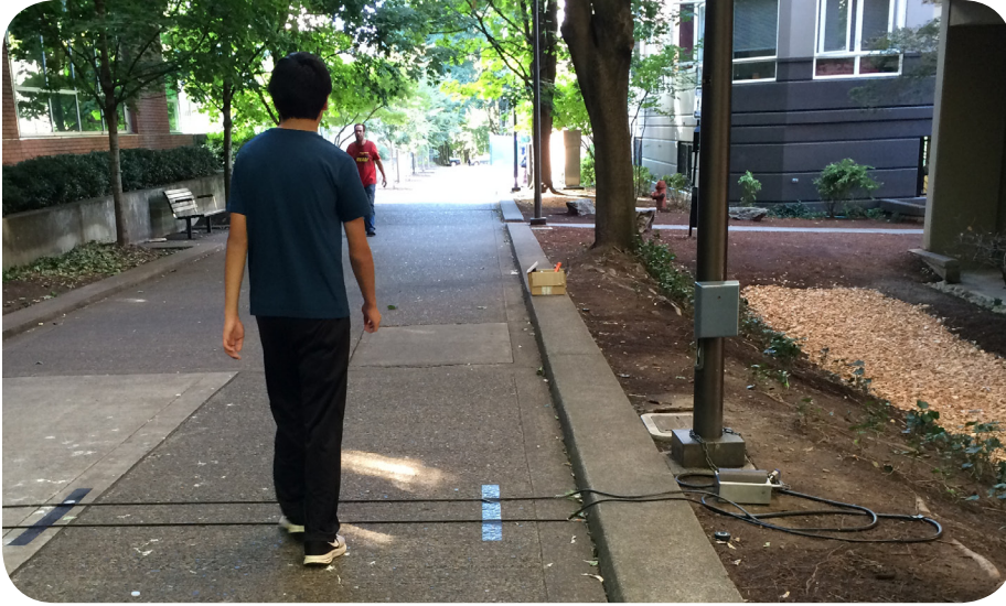
Passive infrared and pneumatic tubes combination
