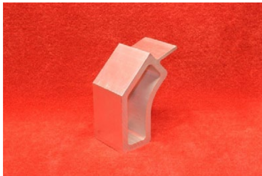
Figure 6-2 A-Pillar custom aluminum extrusion
