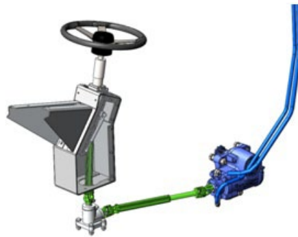
Figure 3-1 CAD of completed steering system
