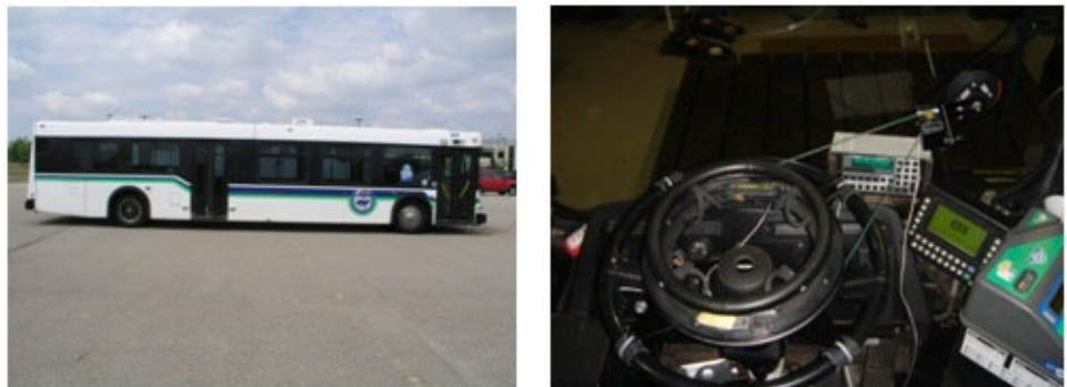
Figure 1-1 Benchmark bus and drivers' area test instrumentation setup
