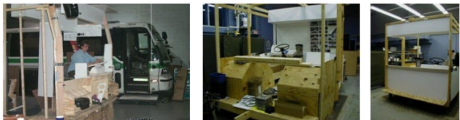
Figure 2-2 Driver's area design space mockup
