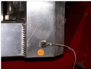
Figure 7-5 Accelerometer setup and geometric point locations
