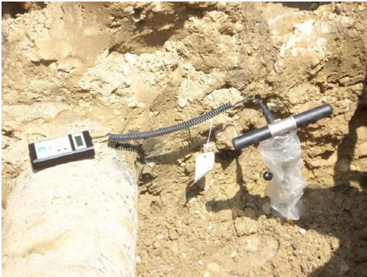
Figure 15 - Corrosion measurement using the LPR Aquamate soil probe
