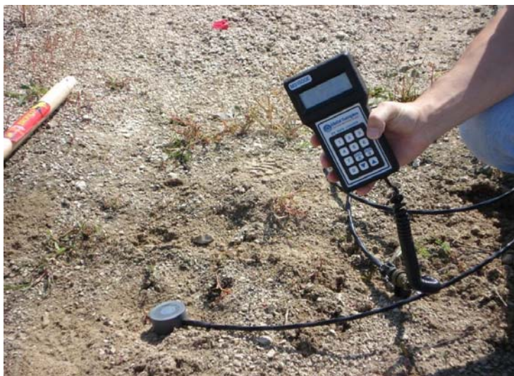
Figure 33 - View of the ER probe and readout box before installation
