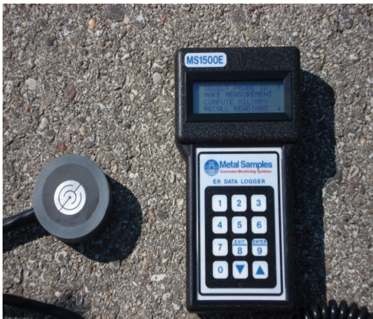
Figure 18 - 'Metal Samples' ER sensor with Flush element and readout box
