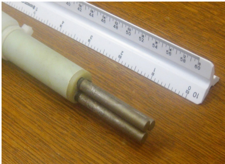
Figure 2 - View of the 3-Electrode LPR probe
