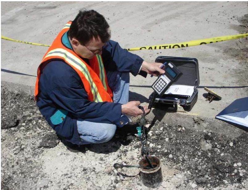
Figure 61 - ER measurements in the Utility-E Site-1
