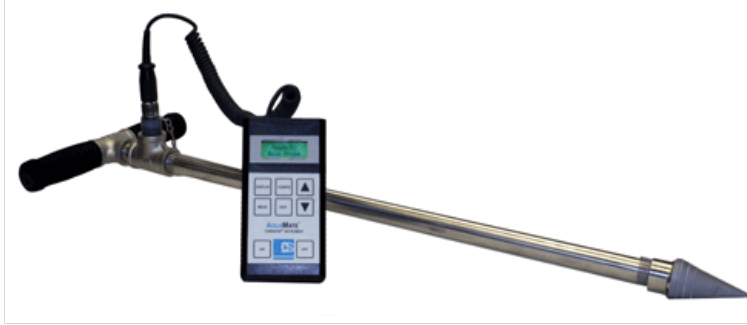
Figure 14 - The portable 'Aquamate Corrat' LPR probe
