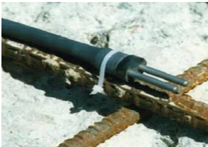
Figure 3 - Commercial LPR probe mounted above rebar
