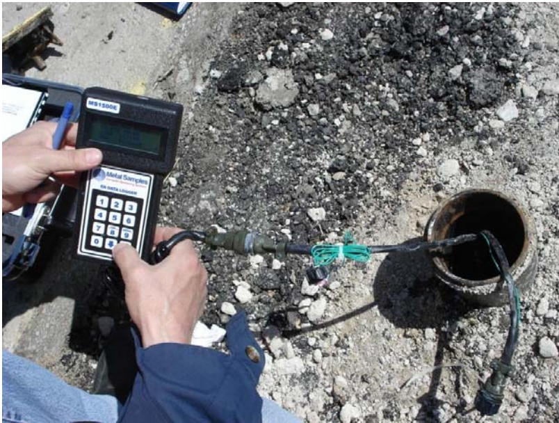
Figure 63 - ER measurement at the Utility-E Site-2
