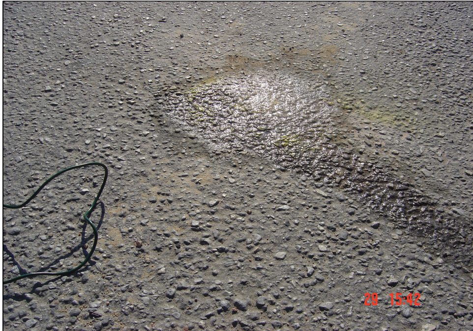
Condition 7: Weathered Concrete/Asphalt Mix Acceptable for Potential Measurements Resistance = 1,100 Ohm-Ft 2
