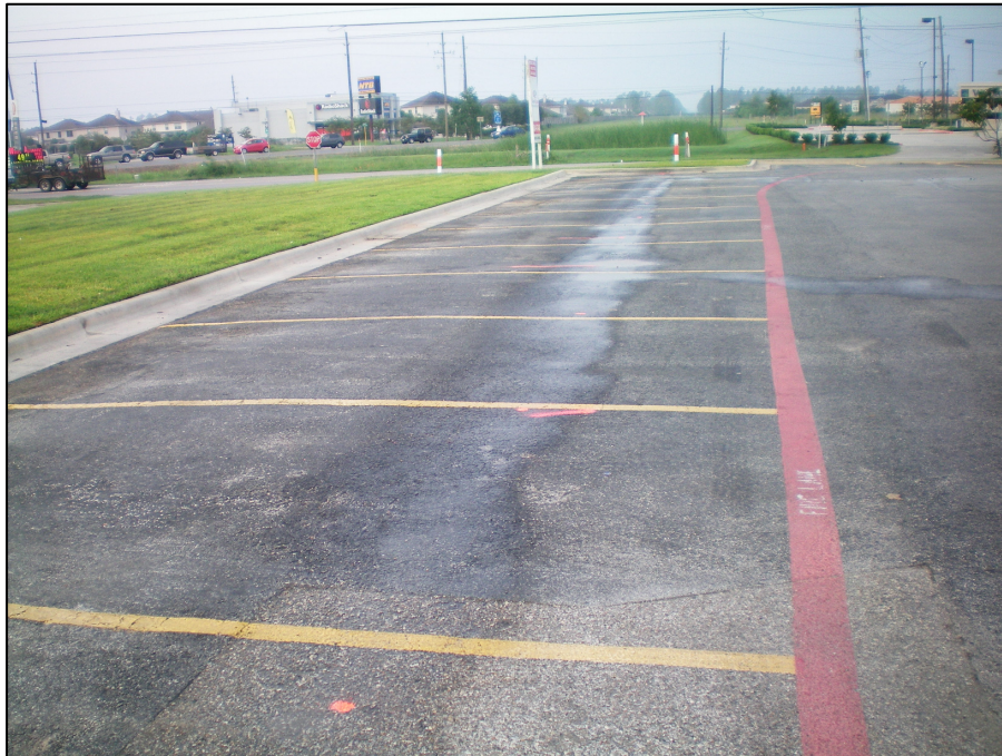
Condition 2: Asphalt (~4 years old) Acceptable for Potential Measurements After Light Surface Wetting Dry Resistance = 10^7 - 10^8 Ohm-Ft 2 Wet Resistance = 10^3 - 10^4 Ohm-Ft 2
