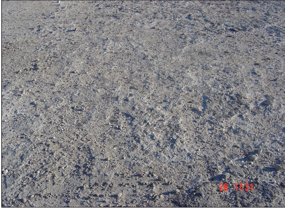
Condition 1: Weathered Asphalt/Rock Acceptable for Potential Measurements Resistance = 49,000 Ohm-Ft 2
