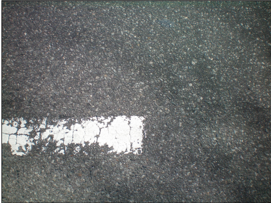
Condition 5: Asphalt Acceptable for Potential Measurements Resistance After Light Surface Wetting = 10^3 - 10^4 Ohm-Ft 2
